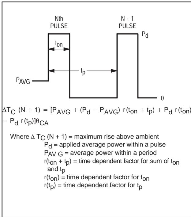
Figure 6.6. Steady State Peak Case Temperature Rise
