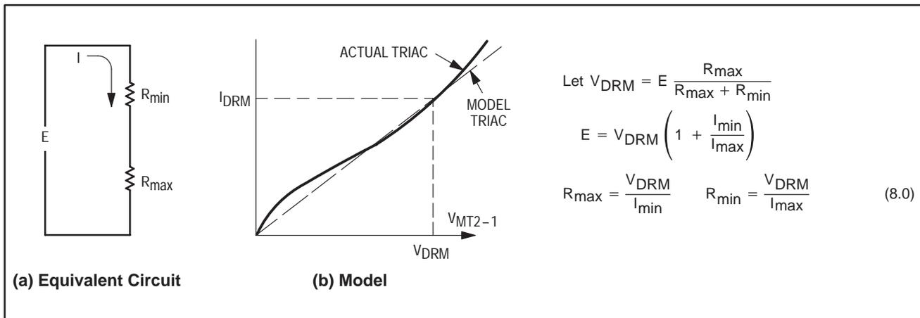
Figure 6.8. Maximum Voltage Sharing Without Shunt Resistor
