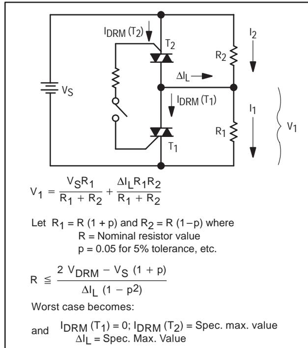
Figure 6.7. Maximum Allowed Resistor for Static Voltage Sharing
