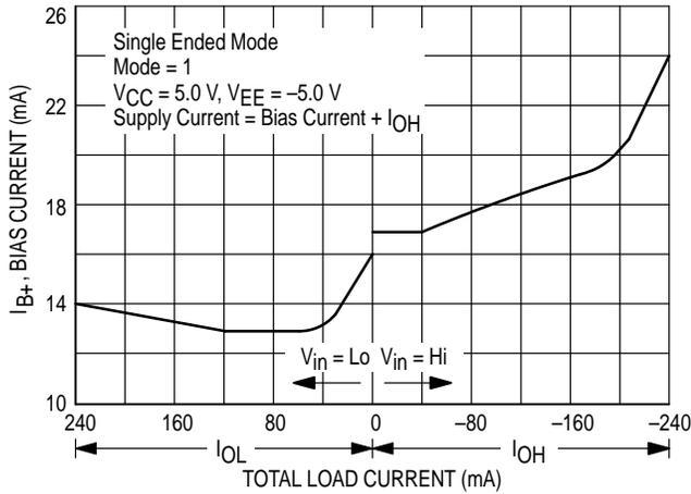
Figure 13. Internal Negative Bias Current versus Load Current
