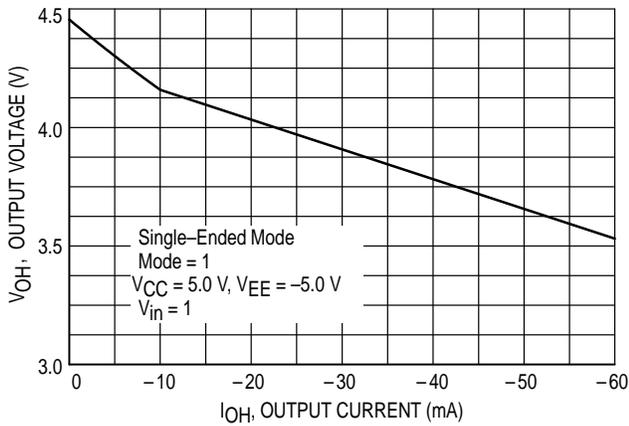
**Figure 11. Output Voltage versus Output Sink Current**
