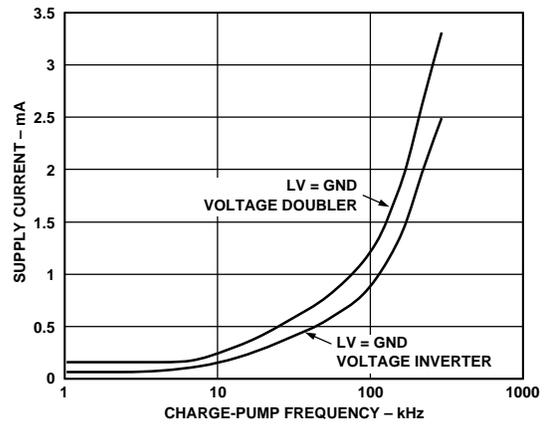
Figure 5. Power Supply Current vs. Charge-Pump Frequency
