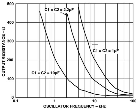
Figure 23. Output Impedance vs. Oscillator Frequency
