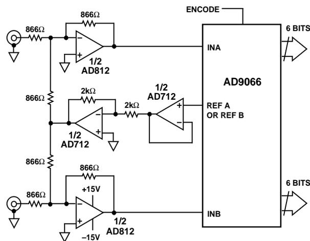
Figure 6. Bipolar Input Using AD812 Drive for AD9066
