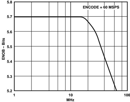
Figure 1. ENOB vs. Analog Input Frequency
