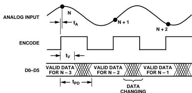
Figure 5. Timing Diagram
