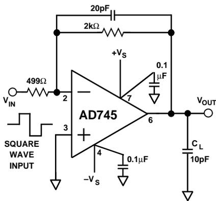
Figure 23a. Gain of 4 Inverter, 8-Pin Package Pinout
