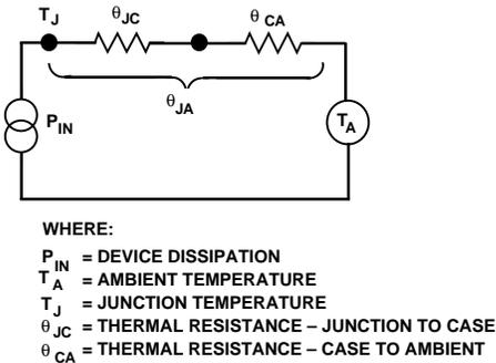
Figure 31. Device Thermal Model
