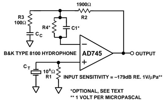
Figure 36a. A Low Noise Hydrophone Amplifier
