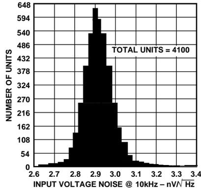
Figure 20. Typical Input Noise Voltage Distribution @ 10 kHz
