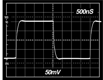
Figure 22c. Gain of 5 Follower Small Signal Pulse Response
