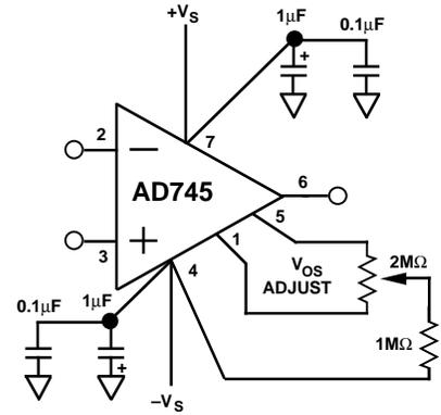
Figure 21. Offset Null Configuration, 8-Pin Package Pinout
