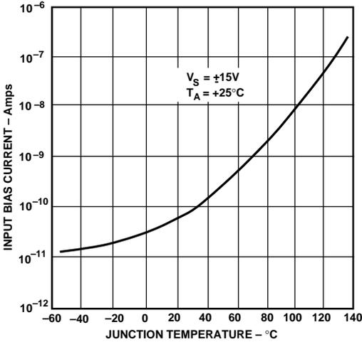
Figure 30. Input Bias Current vs. Junction Temperature
