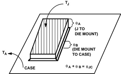
Figure 33. Breakdown of Various Package Thermal Resistance
