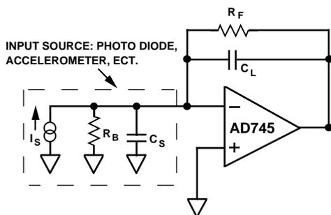
Figure 37. A Model for an I-to-V Converter
