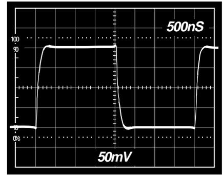
Figure 23c. Gain of 4 Inverter Small Signal Pulse Response
