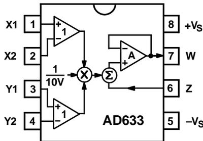
Figure 1. Functional Block Diagram (AD633JN Pinout Shown)
