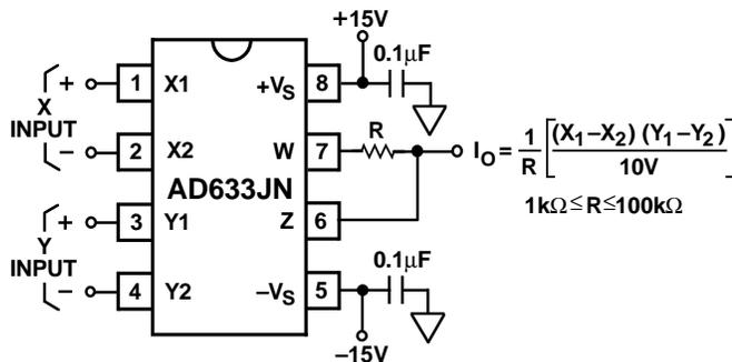
Figure 9. Current Output Connections
