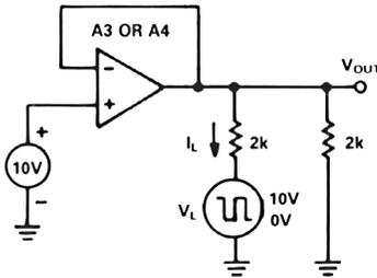
Figure 11a. Transient and Constant Load Test Circuit
