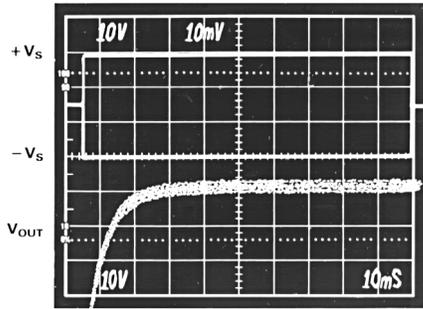
Figure 6. Turn-On with 1 μF C<sub>N</sub>
