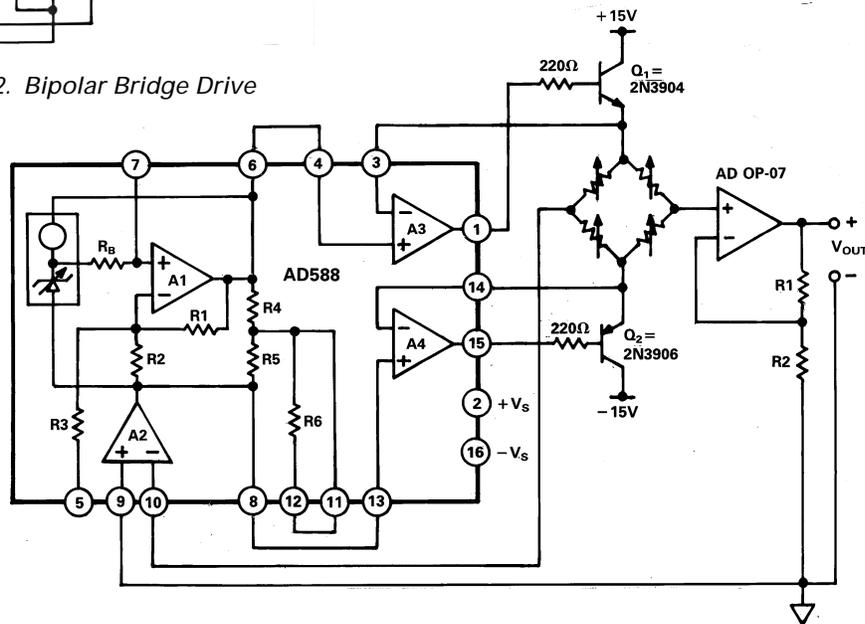
Figure 23. Floating Bipolar Bridge Drive with Minimum CMV
