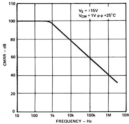
Common-Mode Rejection vs. Frequency (A3, A4)
