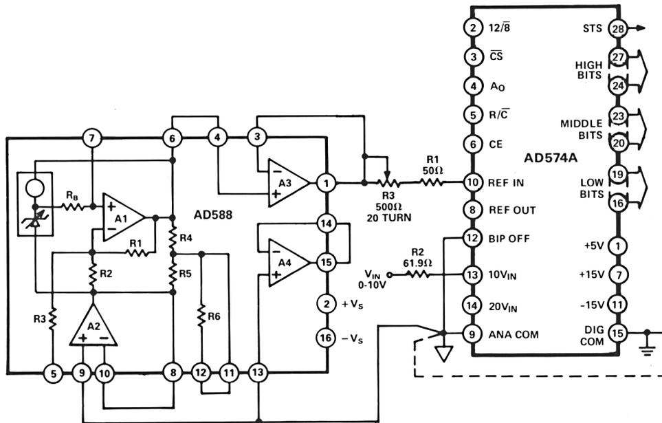
Figure 17. AD588/AD574A Connections
