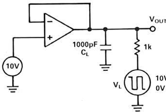
Figure 12a. Capacitive Load Transient Response Test Circuit
