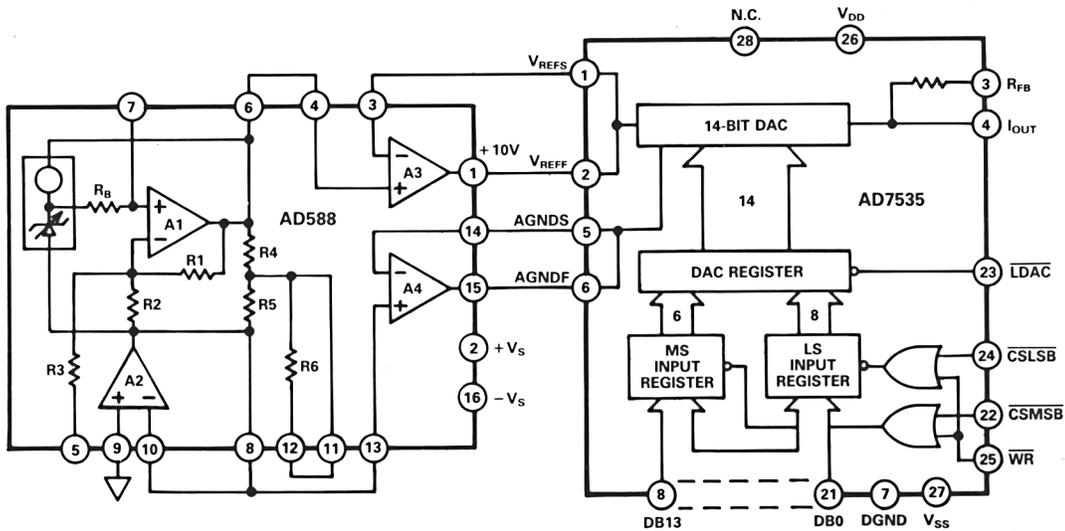
Figure 15. AD588/AD7535 Connections
