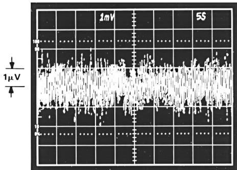
Figure 3. 0.1 Hz to 10 Hz Noise
