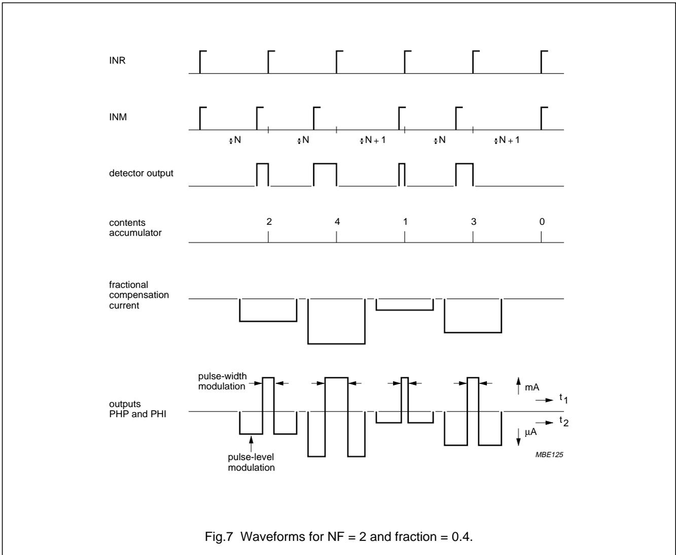
Fig.7 Waveforms for NF = 2 and fraction = 0.4.
