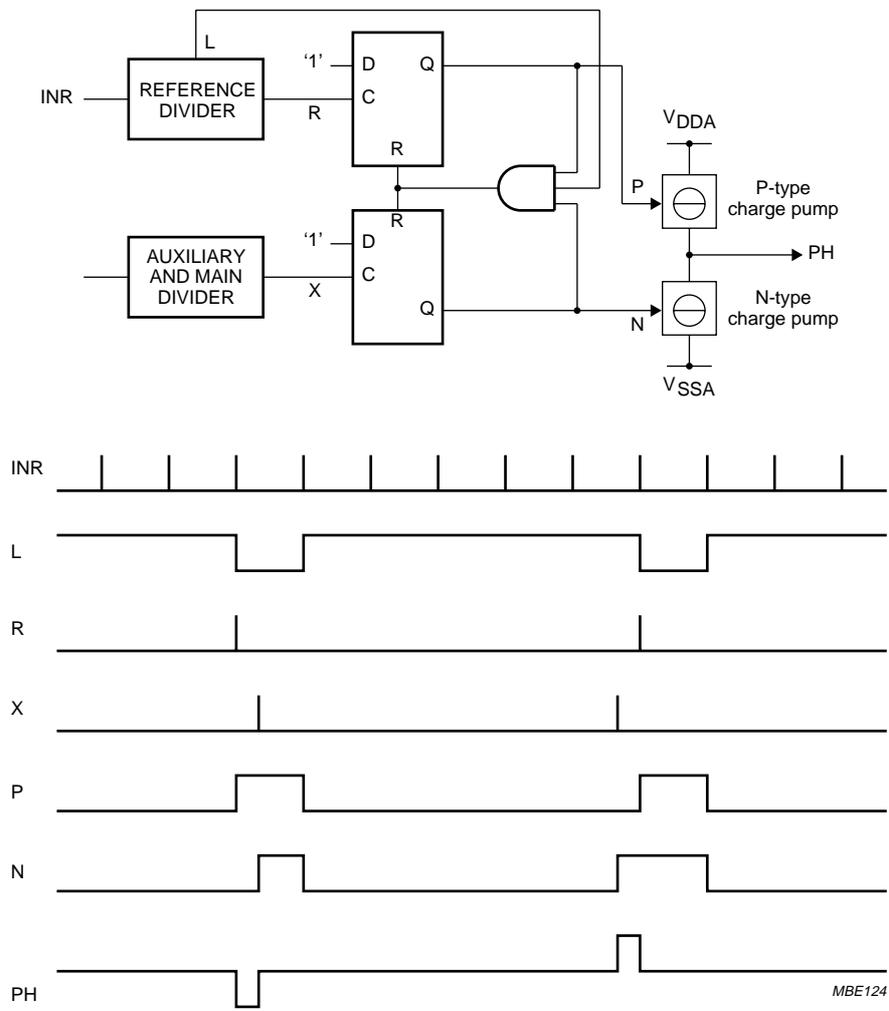
Fig.6 Phase detector structure with timing.
