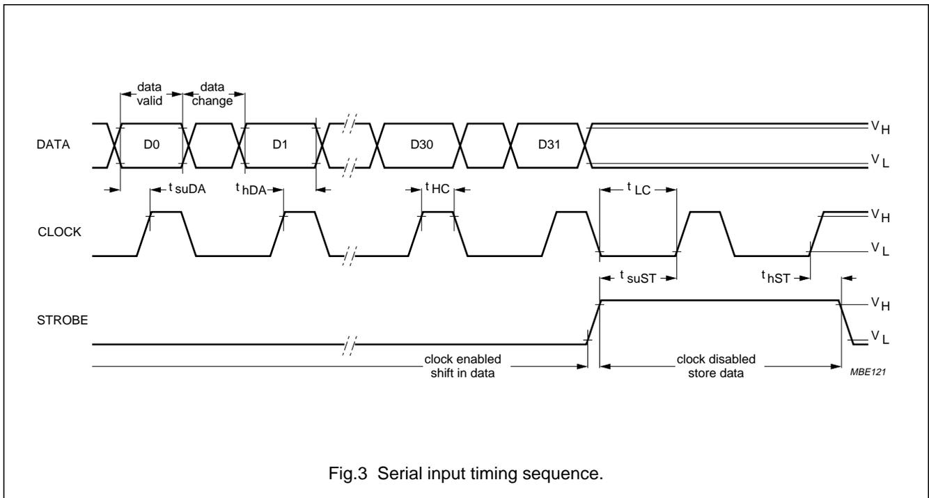
Fig.3 Serial input timing sequence.
