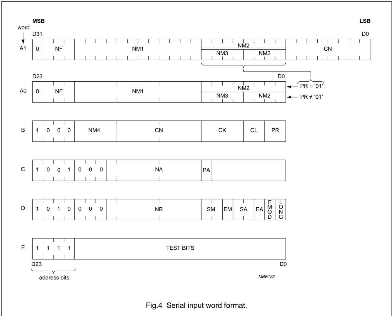
Fig.4 Serial input word format.
