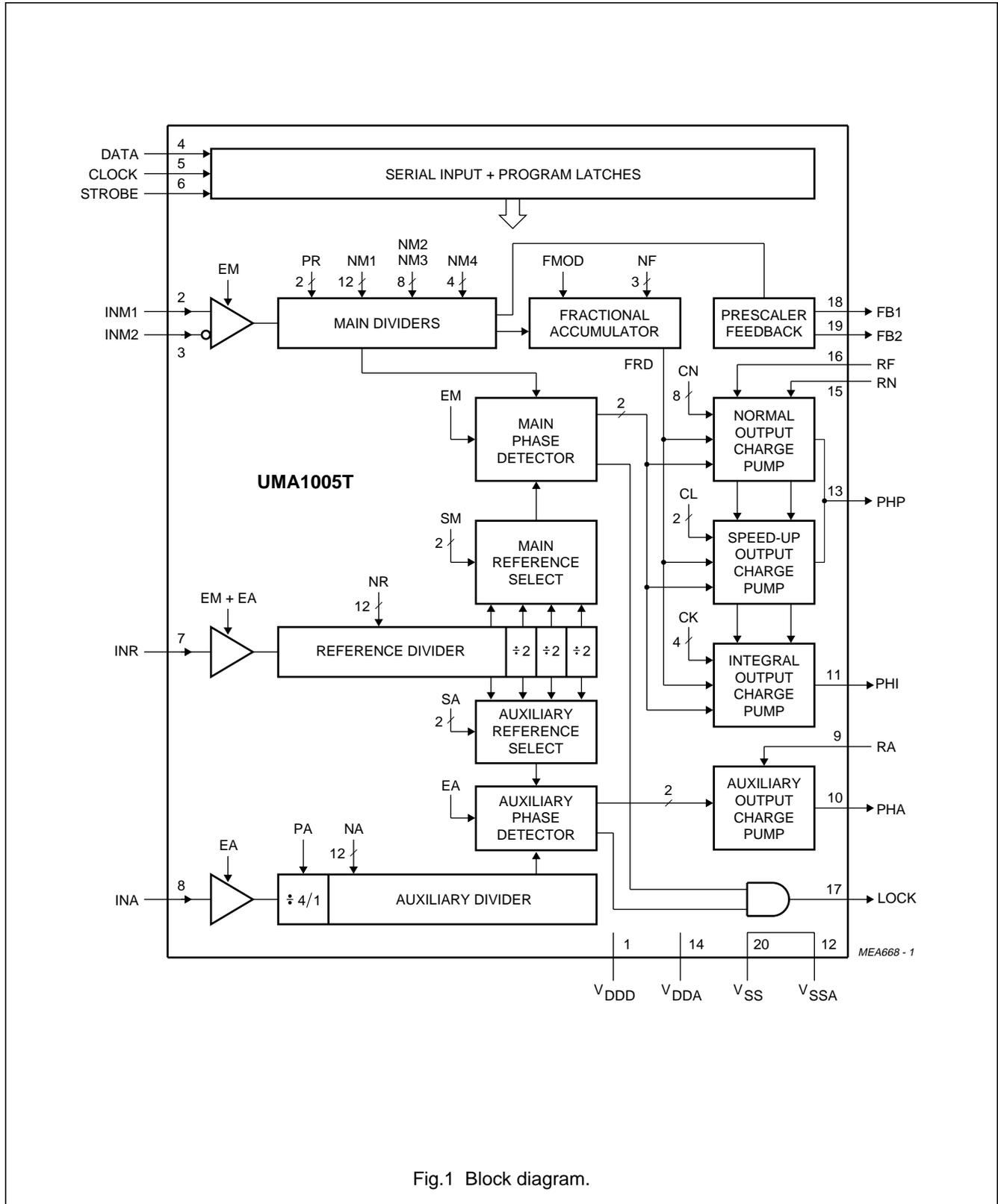
Fig.1 Block diagram.
