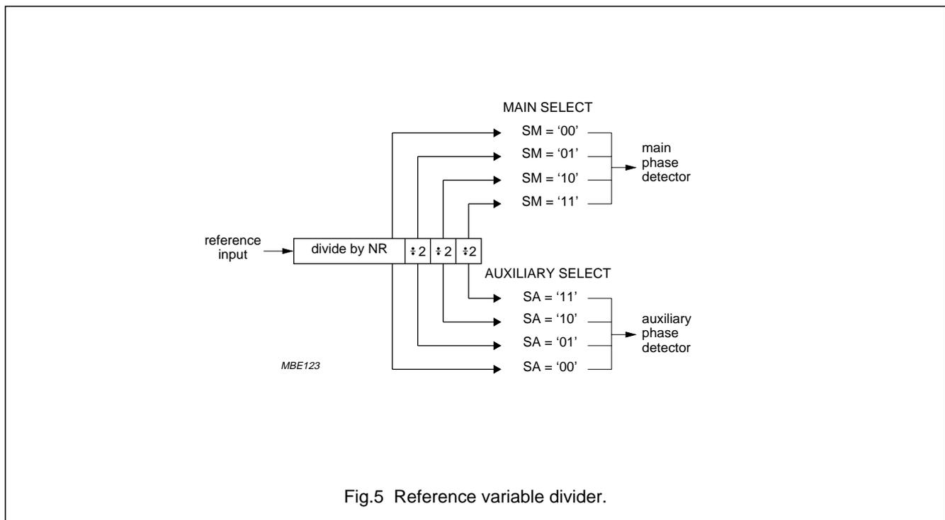
Fig.5 Reference variable divider.
