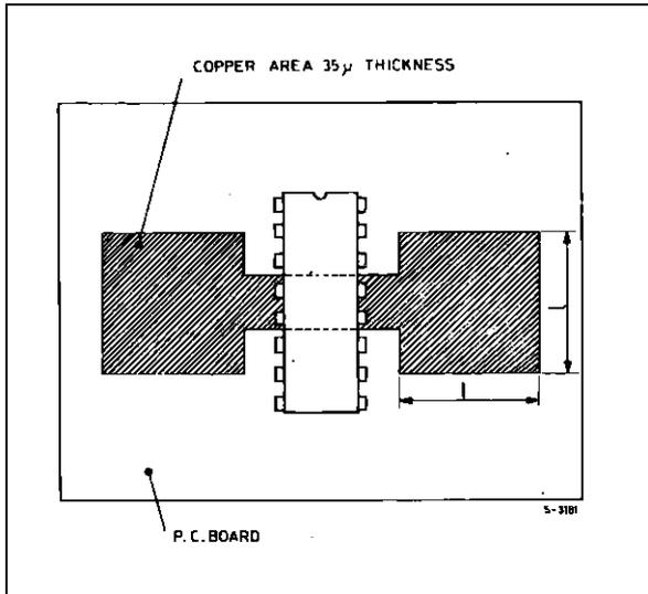
**Figure 13 :** External Heatsink Mounting Example.
