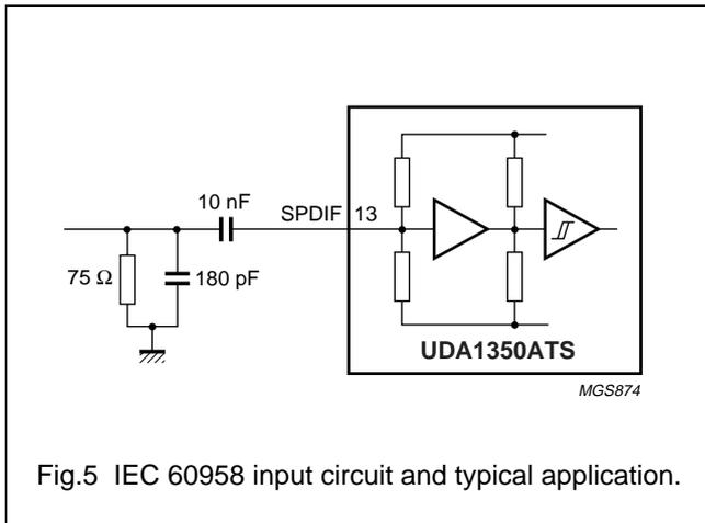
Fig.5 IEC 60958 input circuit and typical application.
