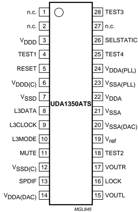
Fig.2 Pin configuration.
