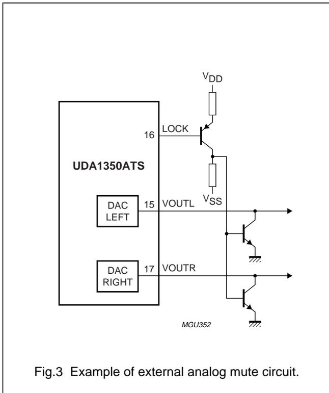
Fig.3 Example of external analog mute circuit.
