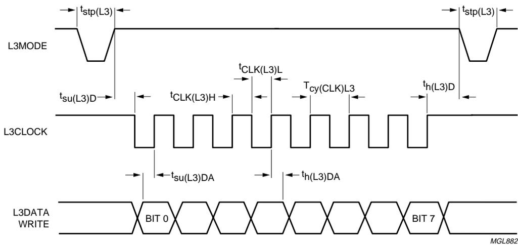
Fig.9 Timing for data transfer mode.
