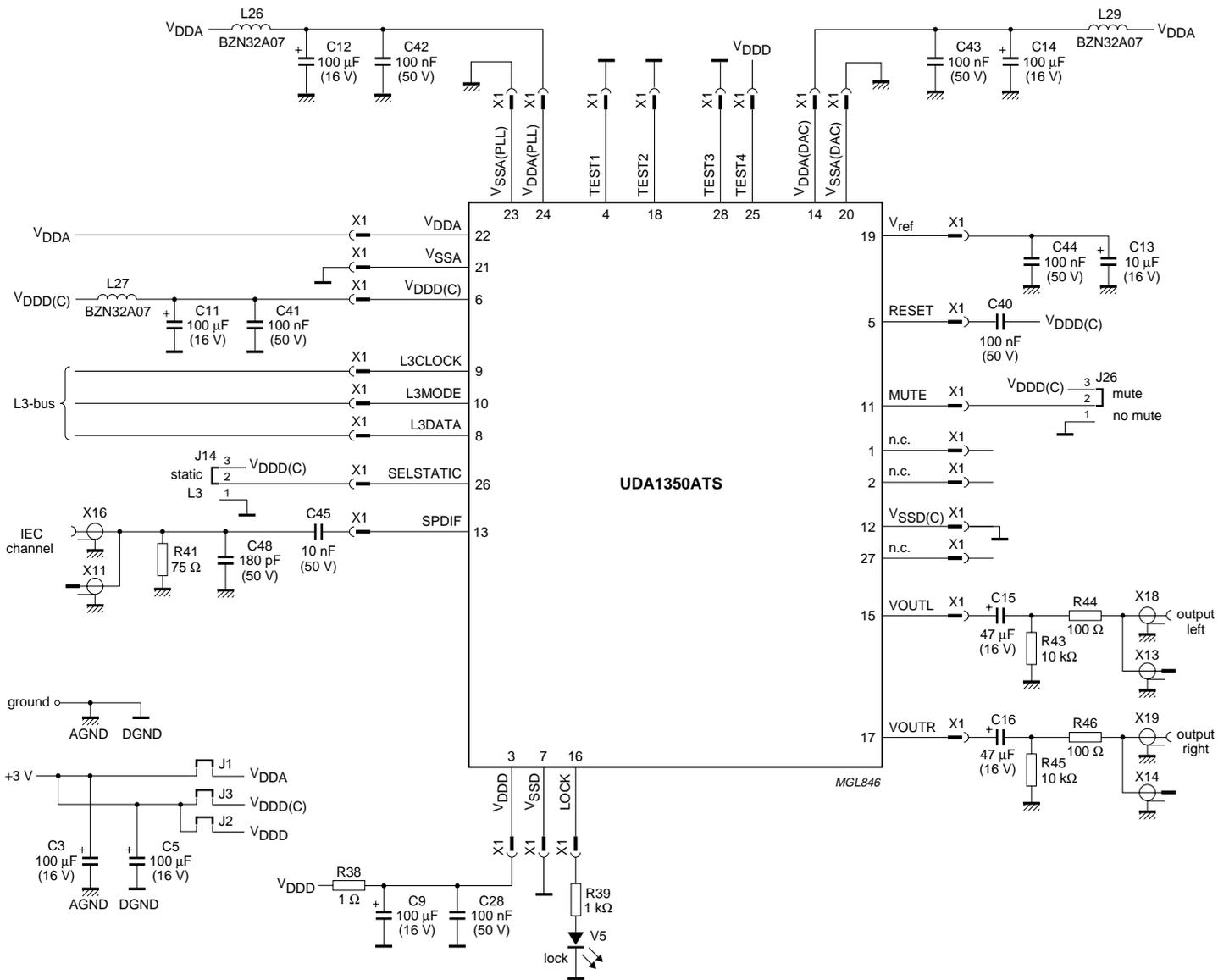
Fig.10 Test and application diagram.
