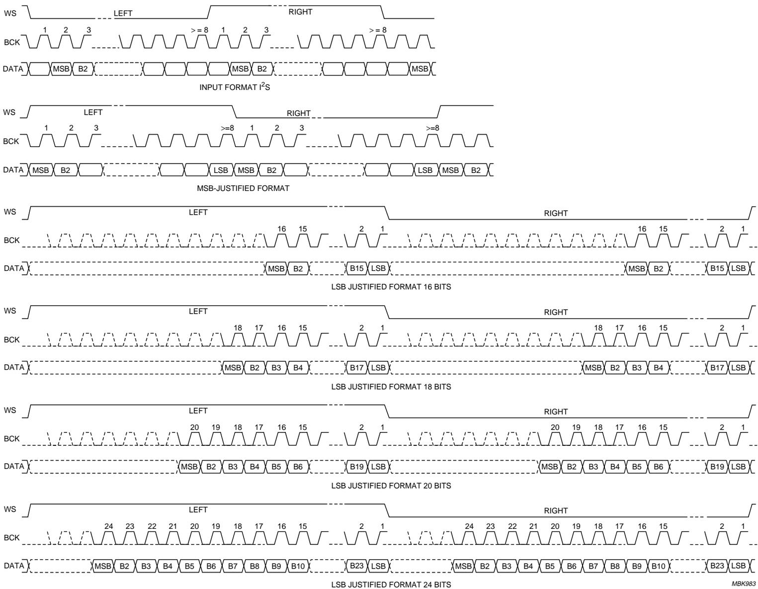
Fig.5 The digital audio interface formats.
