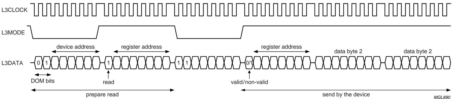
Fig.9 Data read mode for L3 version 2.
