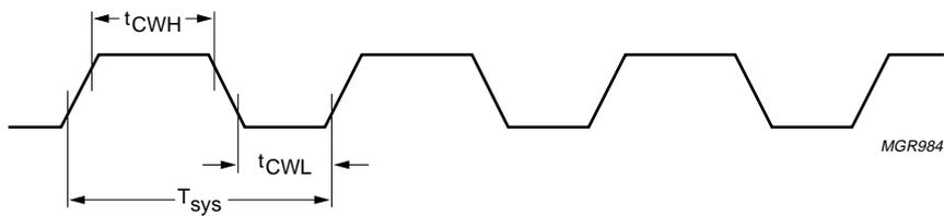
Fig.10 System clock timing.
