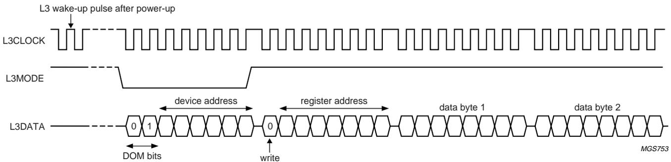
Fig.8 Data write mode for L3 version 2.
