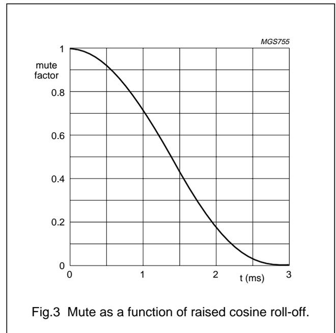
Fig.3 Mute as a function of raised cosine roll-off.
