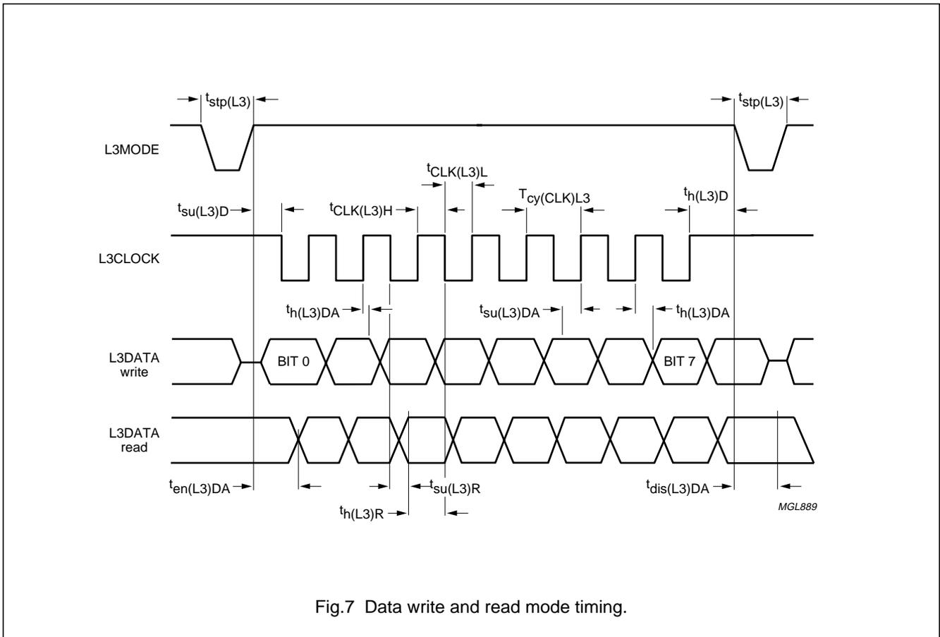
Fig.7 Data write and read mode timing.
