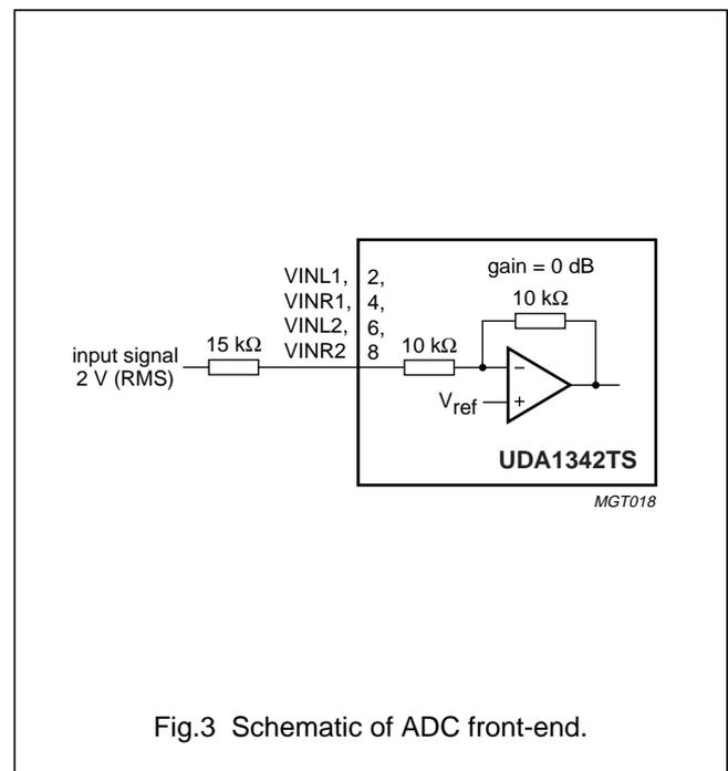
Fig.3 Schematic of ADC front-end.
