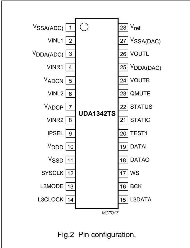
Fig.2 Pin configuration.
