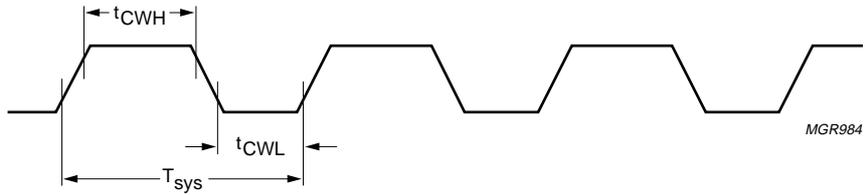
Fig.11 Timing of system clock.
