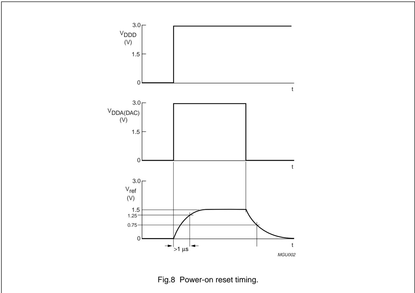
Fig.8 Power-on reset timing.
