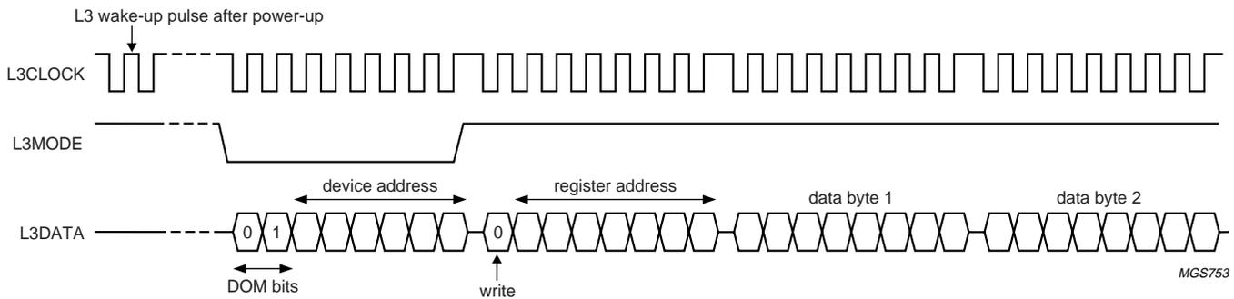
Fig.9 Data write mode for L3-bus version 2.
