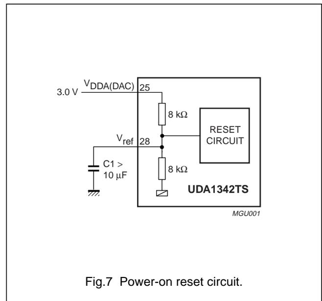
Fig.7 Power-on reset circuit.
