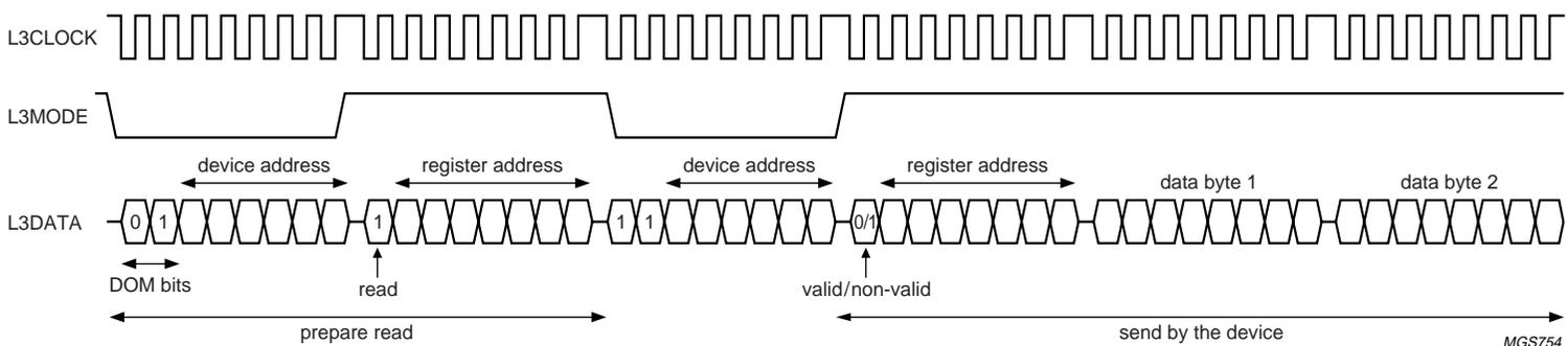
Fig.10 Data read mode for L3-bus version 2.
