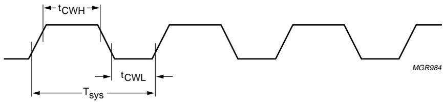
Fig.7 System clock timing.
