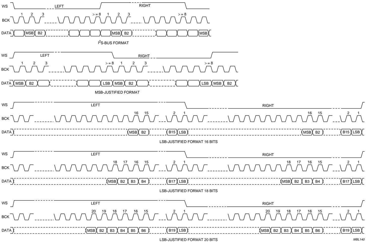
Fig.0 Digital interface input format data format.
