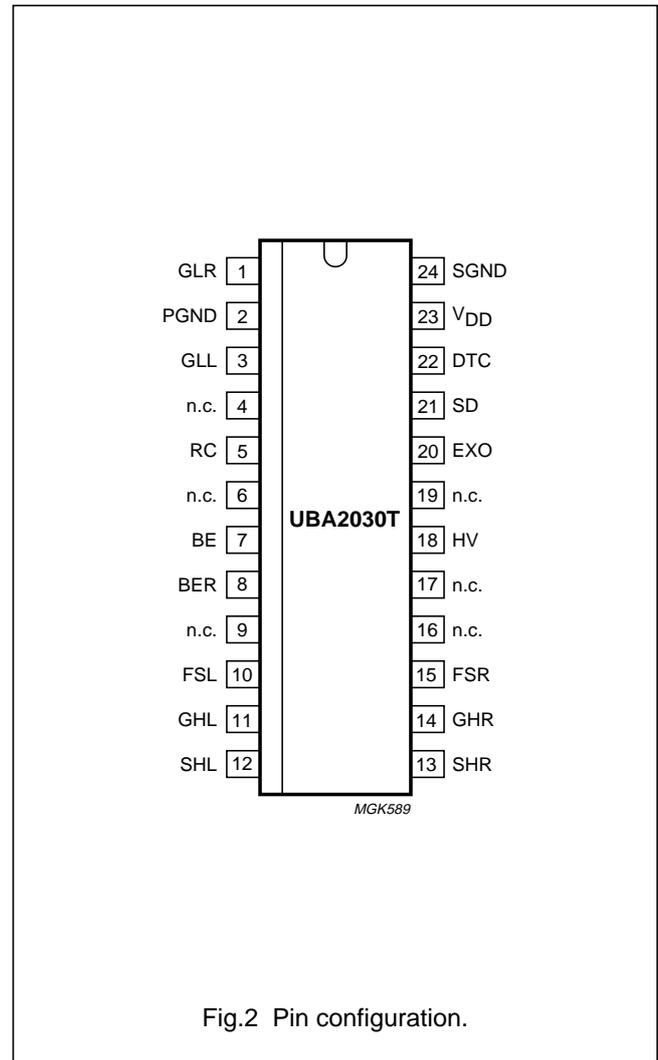
Fig.2 Pin configuration.
