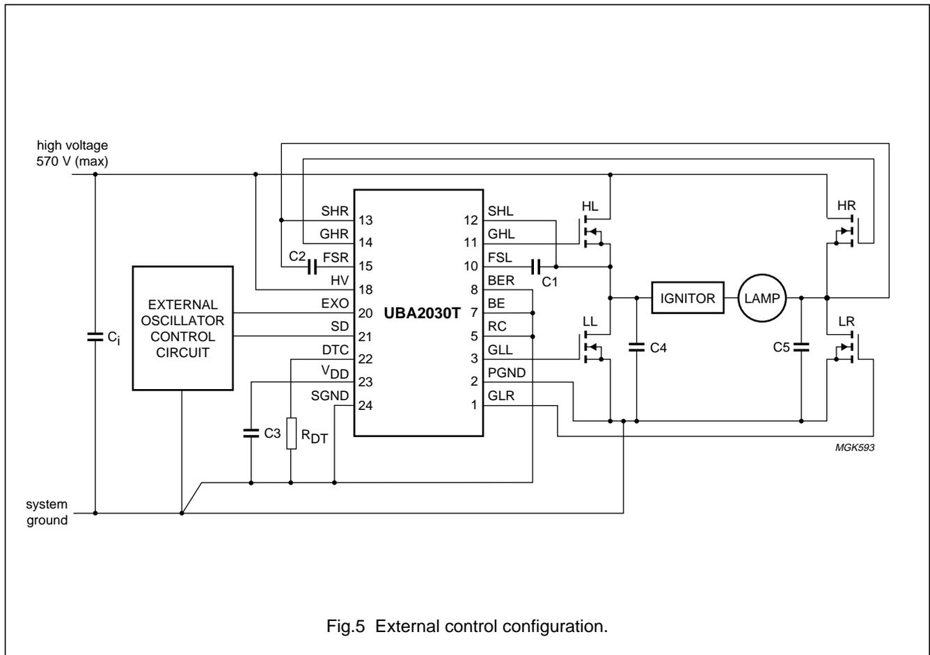
Fig.5 External control configuration.
