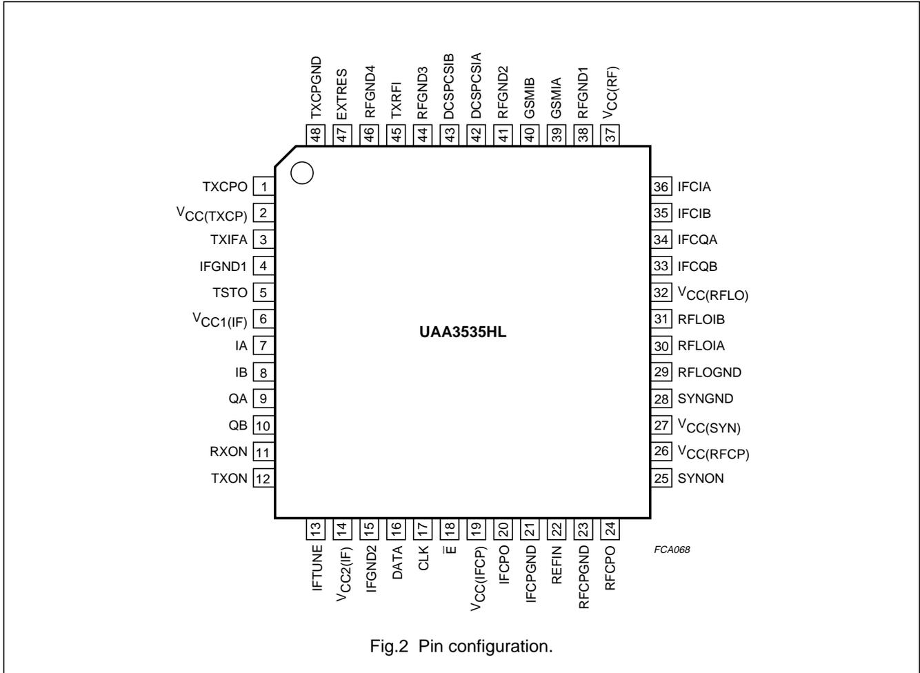
Fig.2 Pin configuration.
