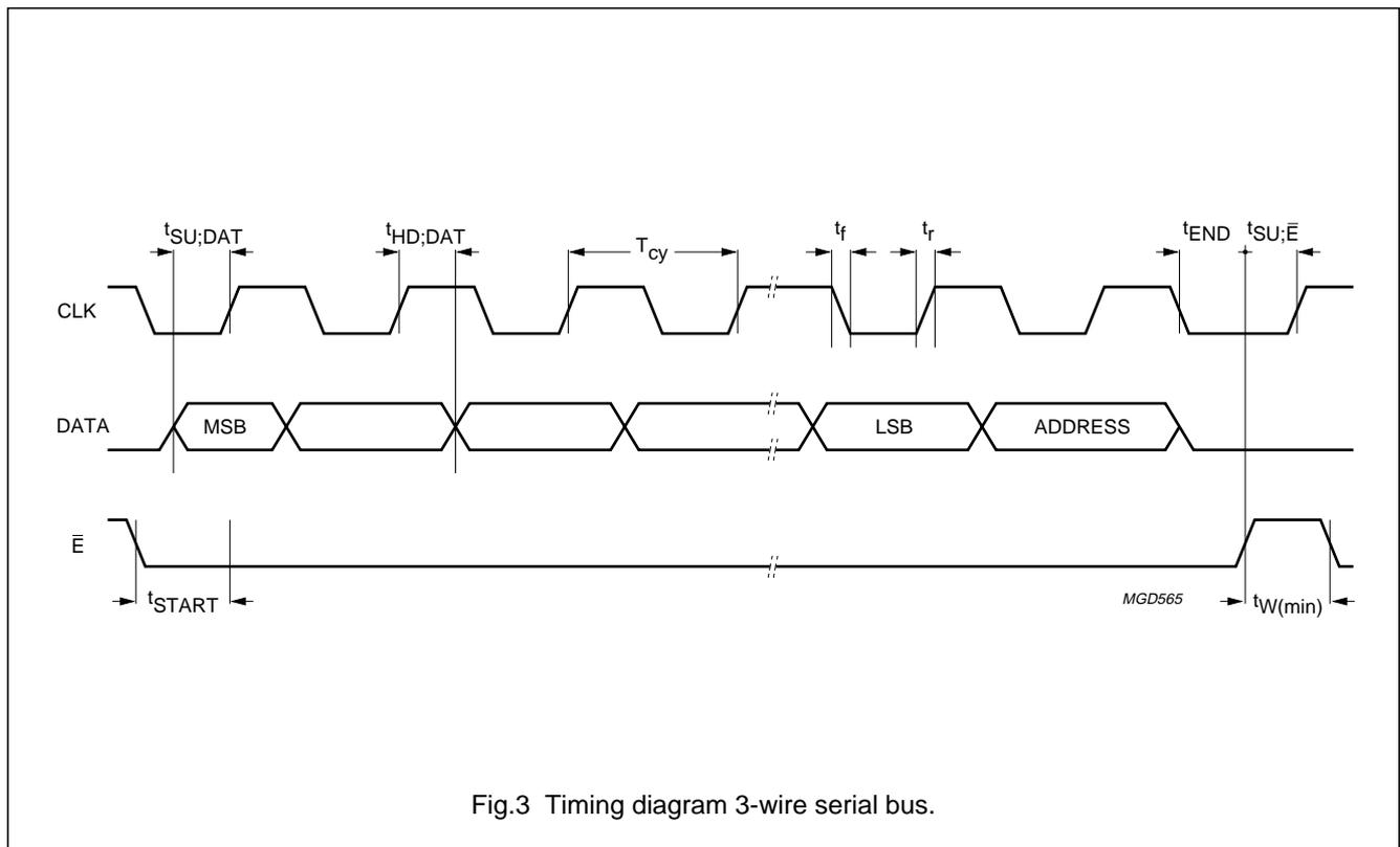
Fig.3 Timing diagram 3-wire serial bus.
