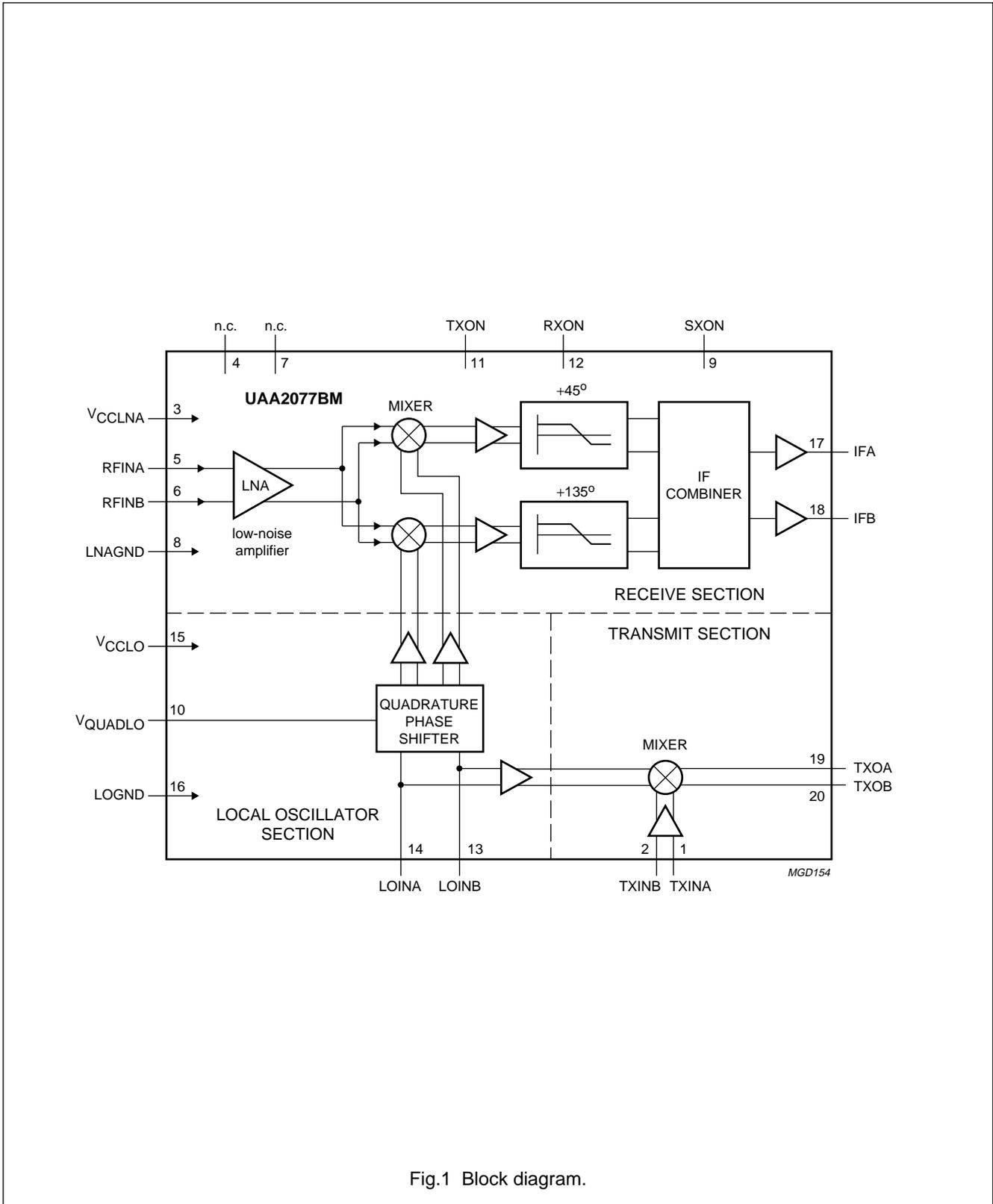
Fig.1 Block diagram.
