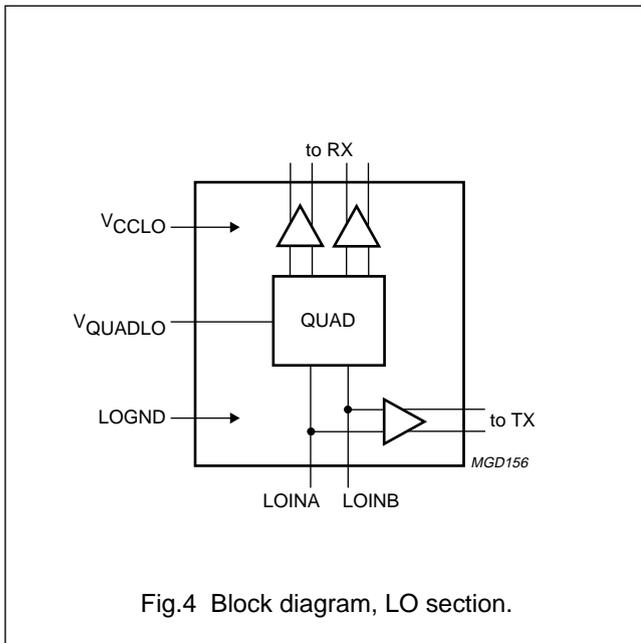
Fig.4 Block diagram, LO section.
