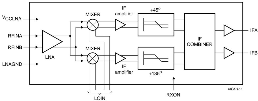
Fig.3 Block diagram, receive section.
