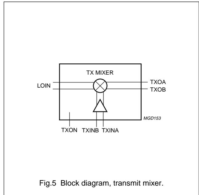
Fig.5 Block diagram, transmit mixer.
