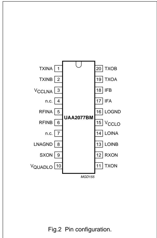
Fig.2 Pin configuration.
