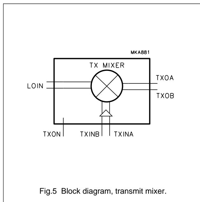
Fig.5 Block diagram, transmit mixer.
