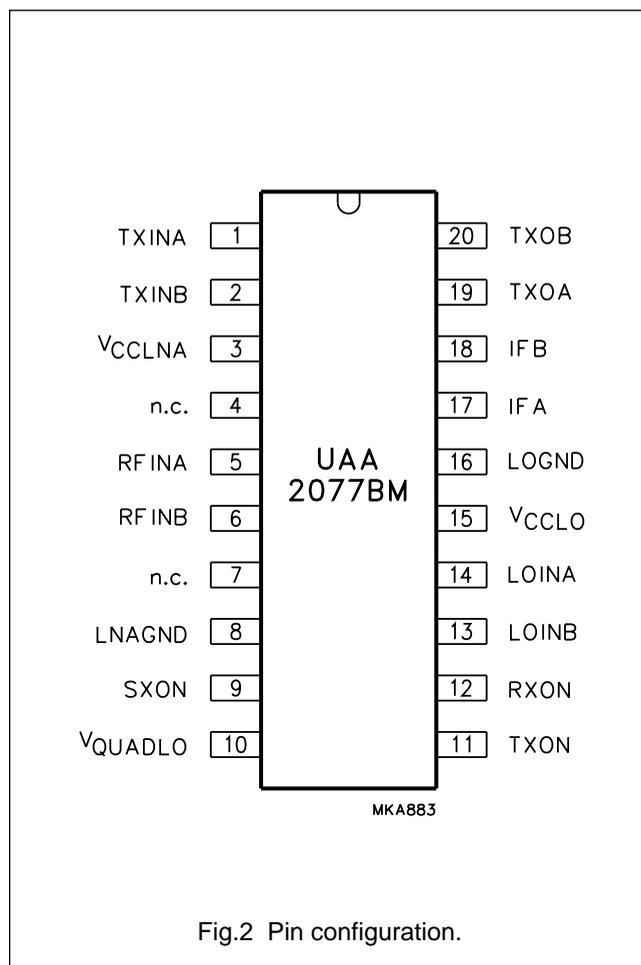
Fig.2 Pin configuration.
