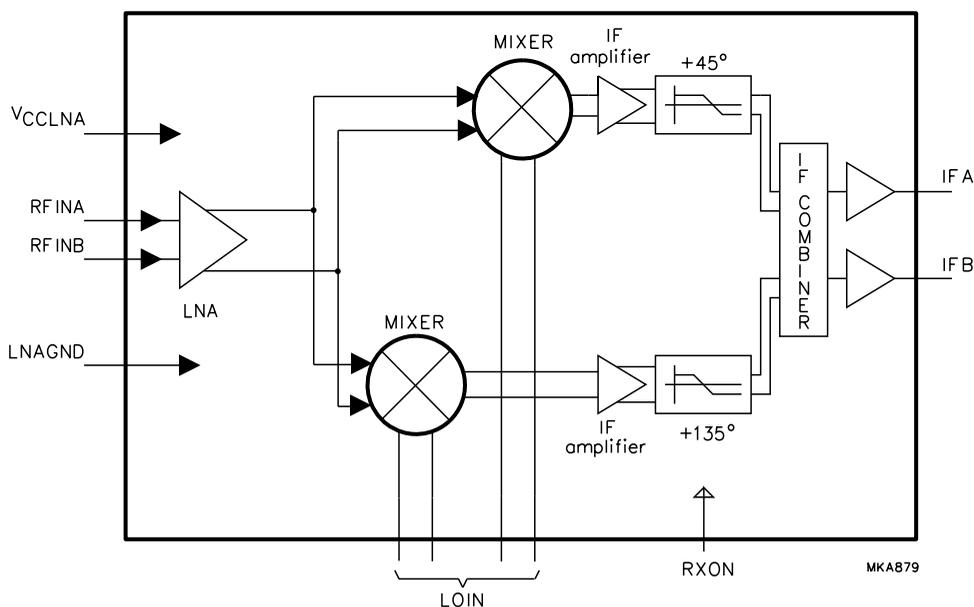
Fig.3 Block diagram, receive section.
