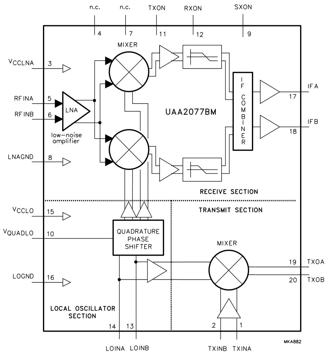
Fig.1 Block diagram.
