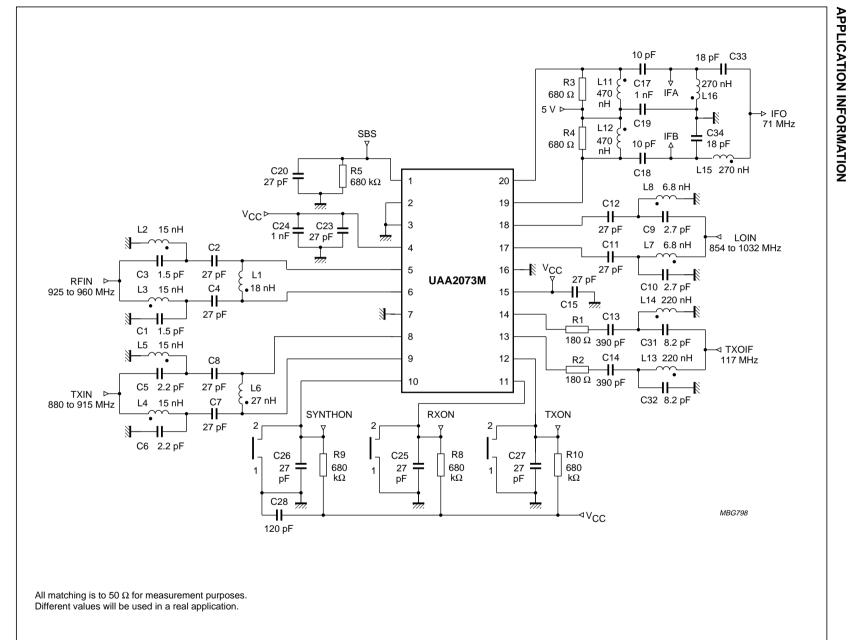
Fig.6 Philips demonstration board diagram for GSM applications.
