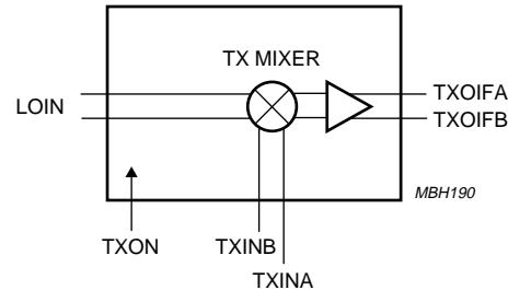
Fig.5 Block diagram, transmit mixer.
