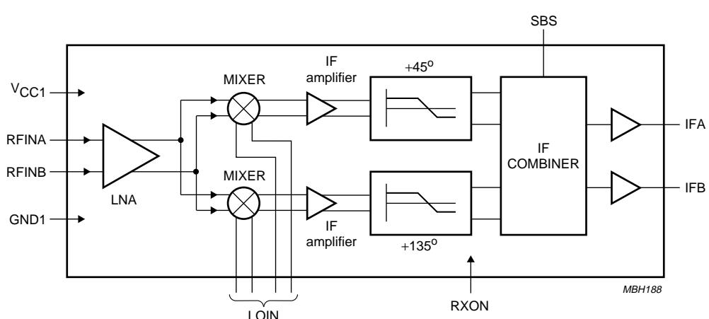
Fig.3 Block diagram, receive section.
