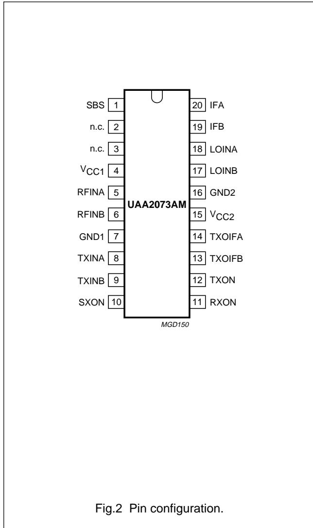
Fig.2 Pin configuration.
