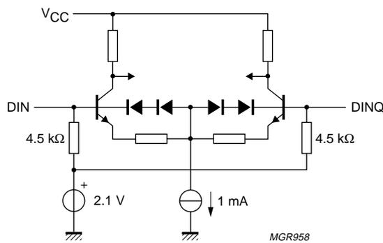
Fig.5 Data input circuit DIN and DINQ.
