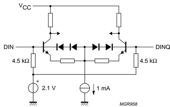
Fig.5 Data input circuit DIN and DINQ.
