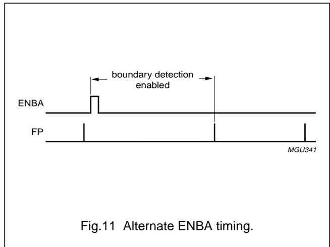
Fig.11 Alternate ENBA timing.
