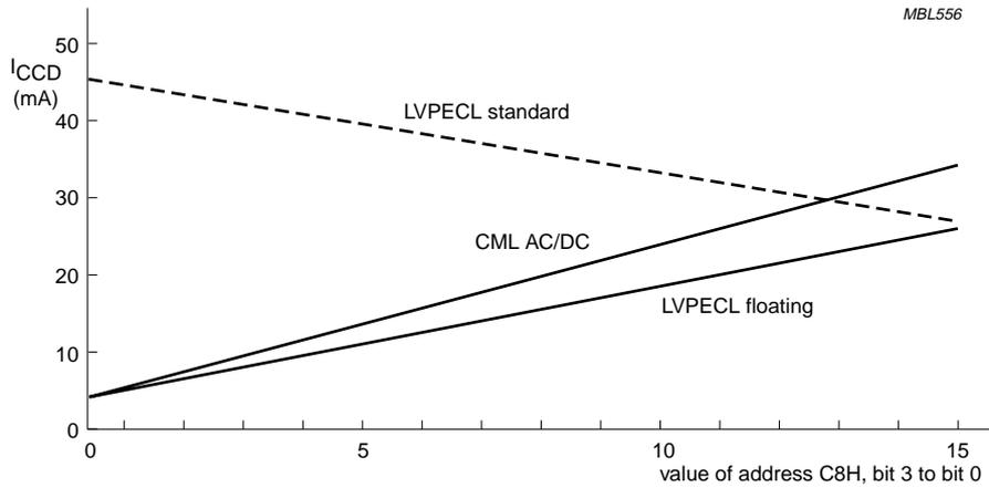
Fig.12 Supply current per parallel output.
