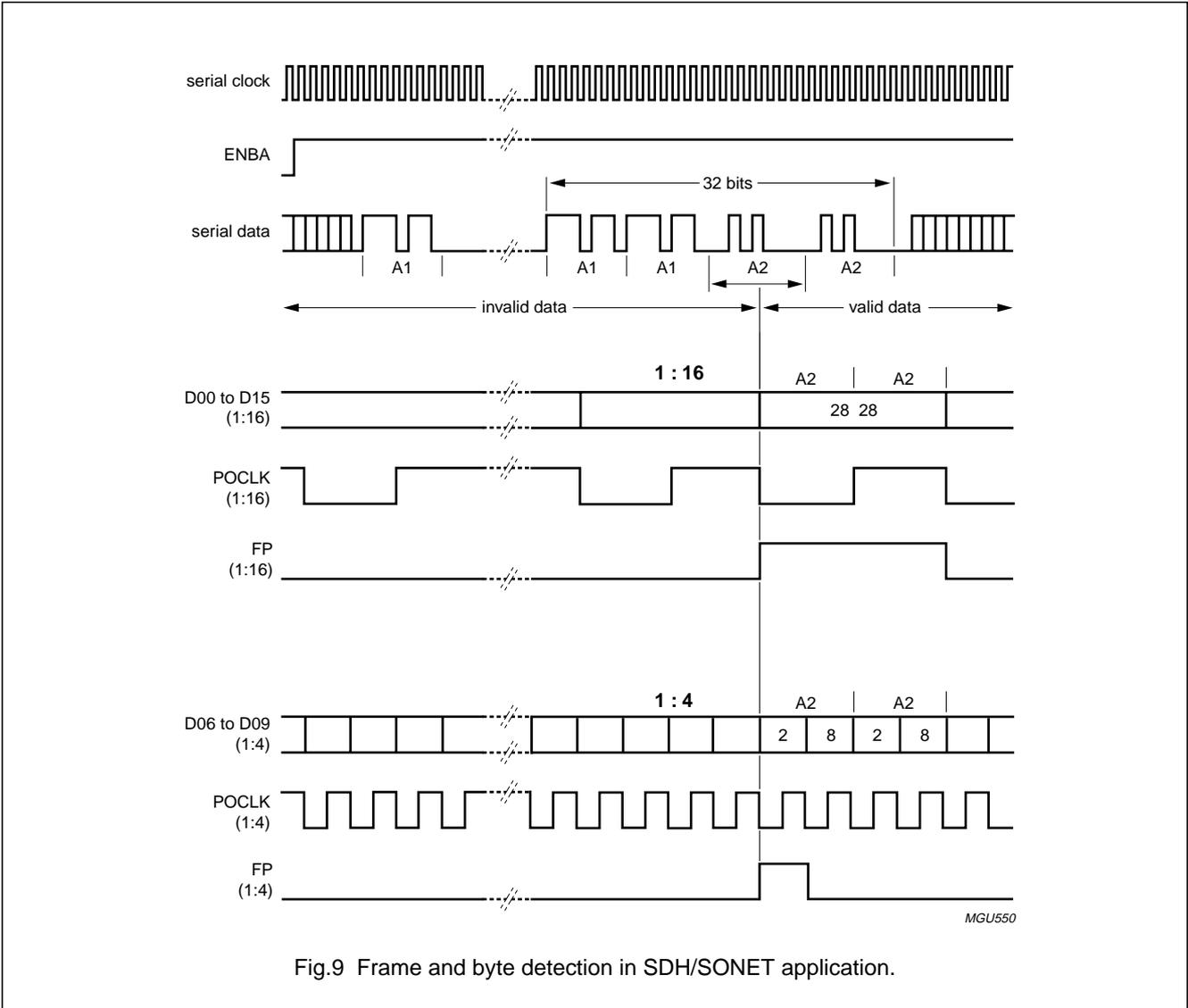
Fig.9 Frame and byte detection in SDH/SONET application.
