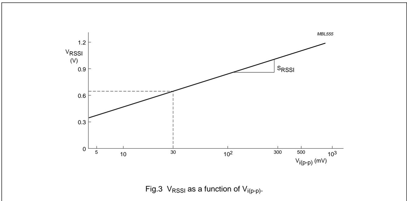
Fig.3 V<sub>RSSI</sub> as a function of V<sub>i(p-p)</sub>.
