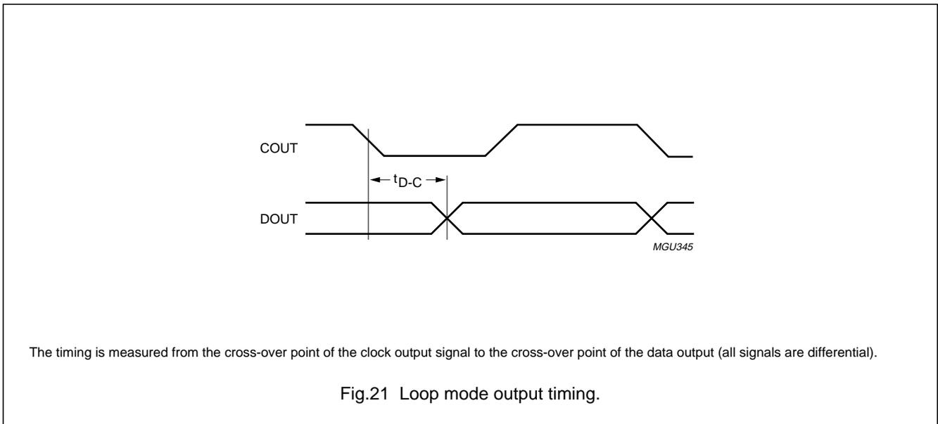
The timing is measured from the cross-over point of the clock output signal to the cross-over point of the data output (all signals are differential).
