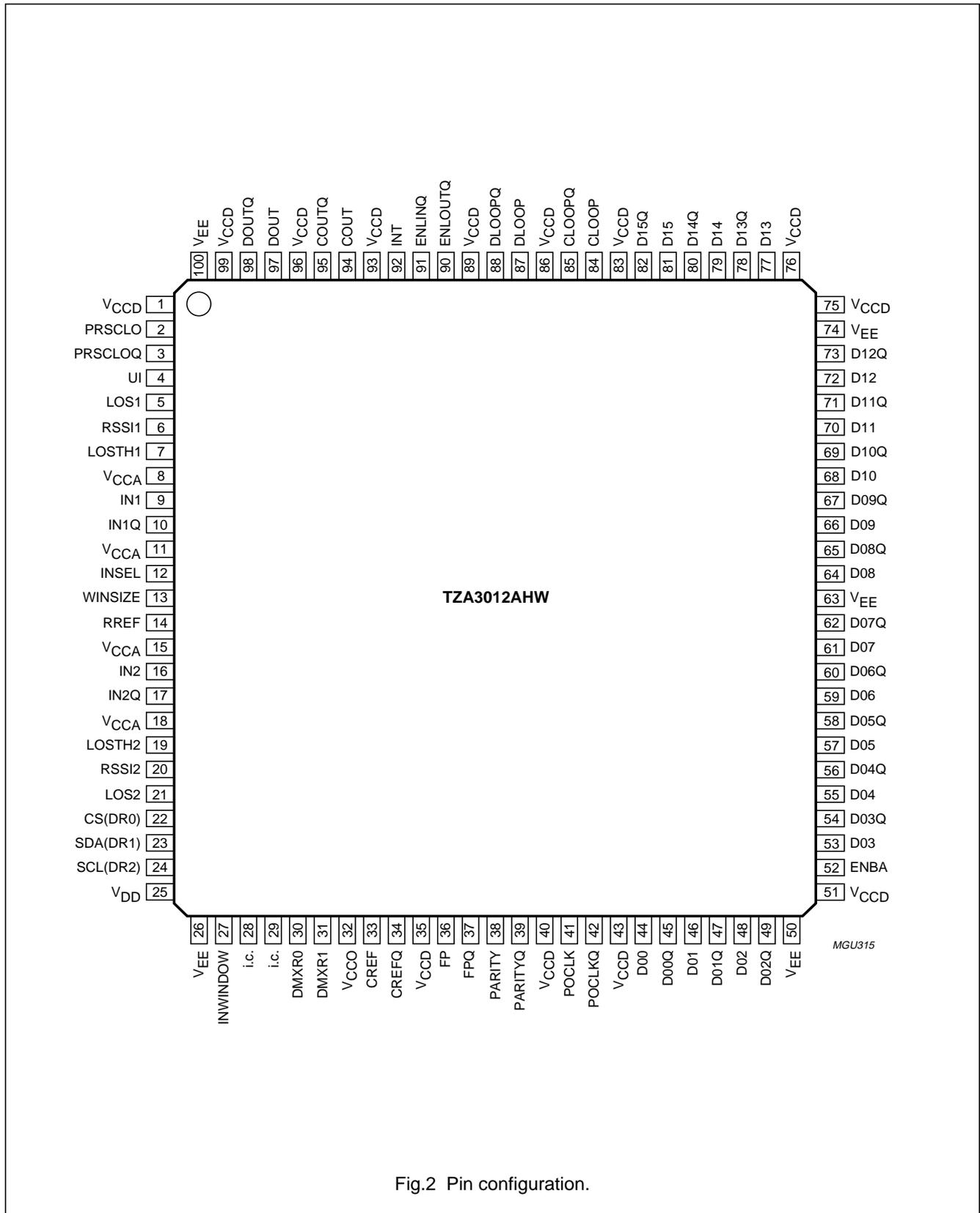
Fig.2 Pin configuration.
