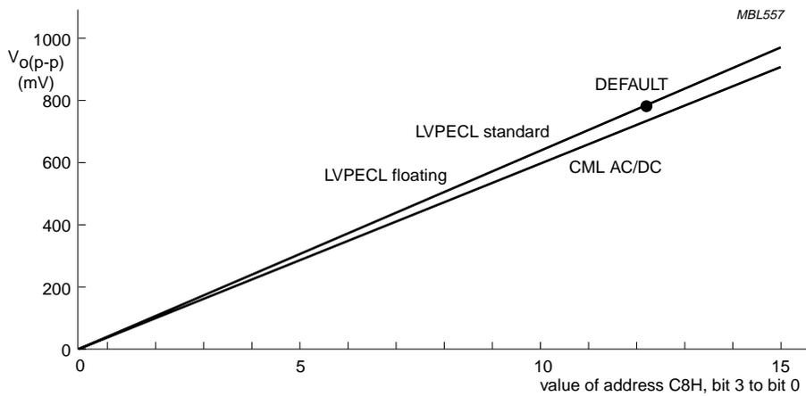
Fig.13 Output voltage swing of parallel output.
