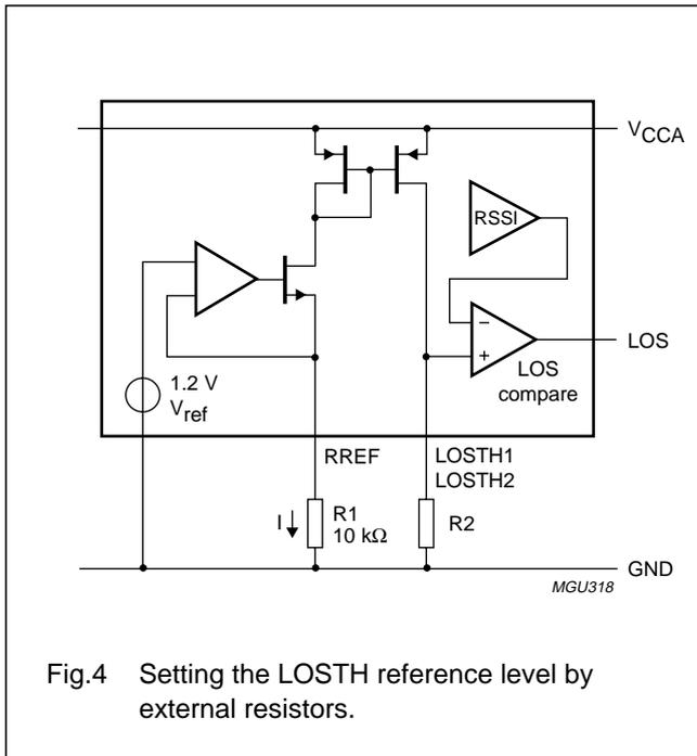
Fig.4 Setting the LOSTH reference level by external resistors.
