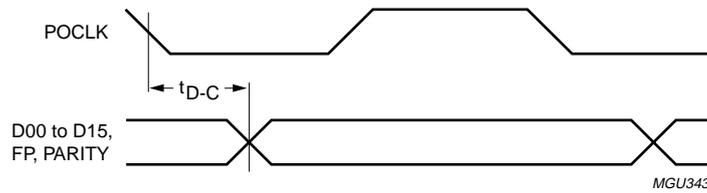
The timing is measured from the cross-over point of the clock output signal to the cross-over point of the data output (all signals are differential).
