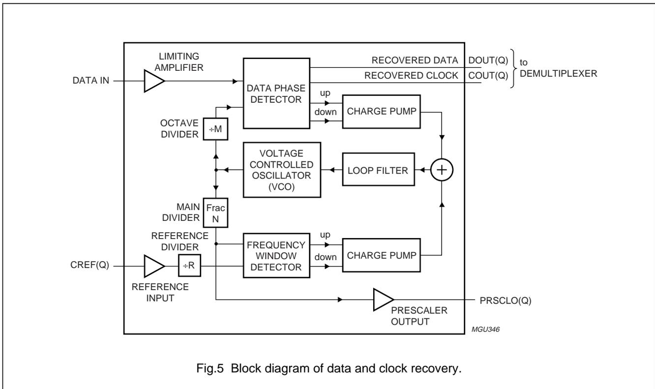
Fig.5 Block diagram of data and clock recovery.
