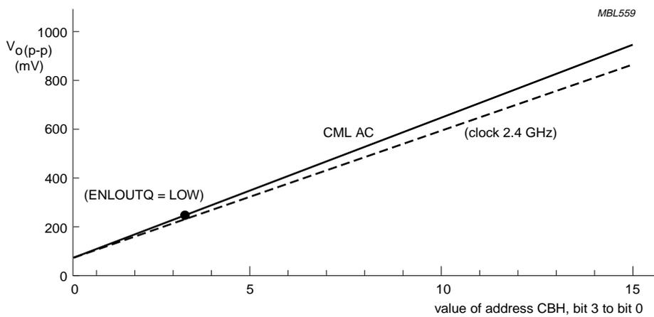
Fig.15 Output voltage swing of serial output.
