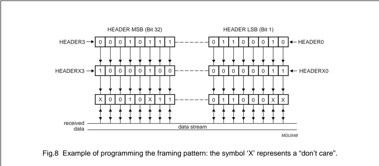
Fig.8 Example of programming the framing pattern: the symbol 'X' represents a "don't care".
