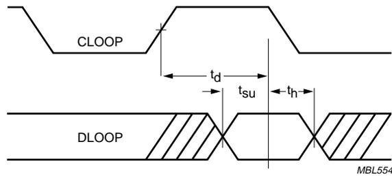
The timing is measured from the cross-over point of the clock input signal to the cross-over point of the data input.
