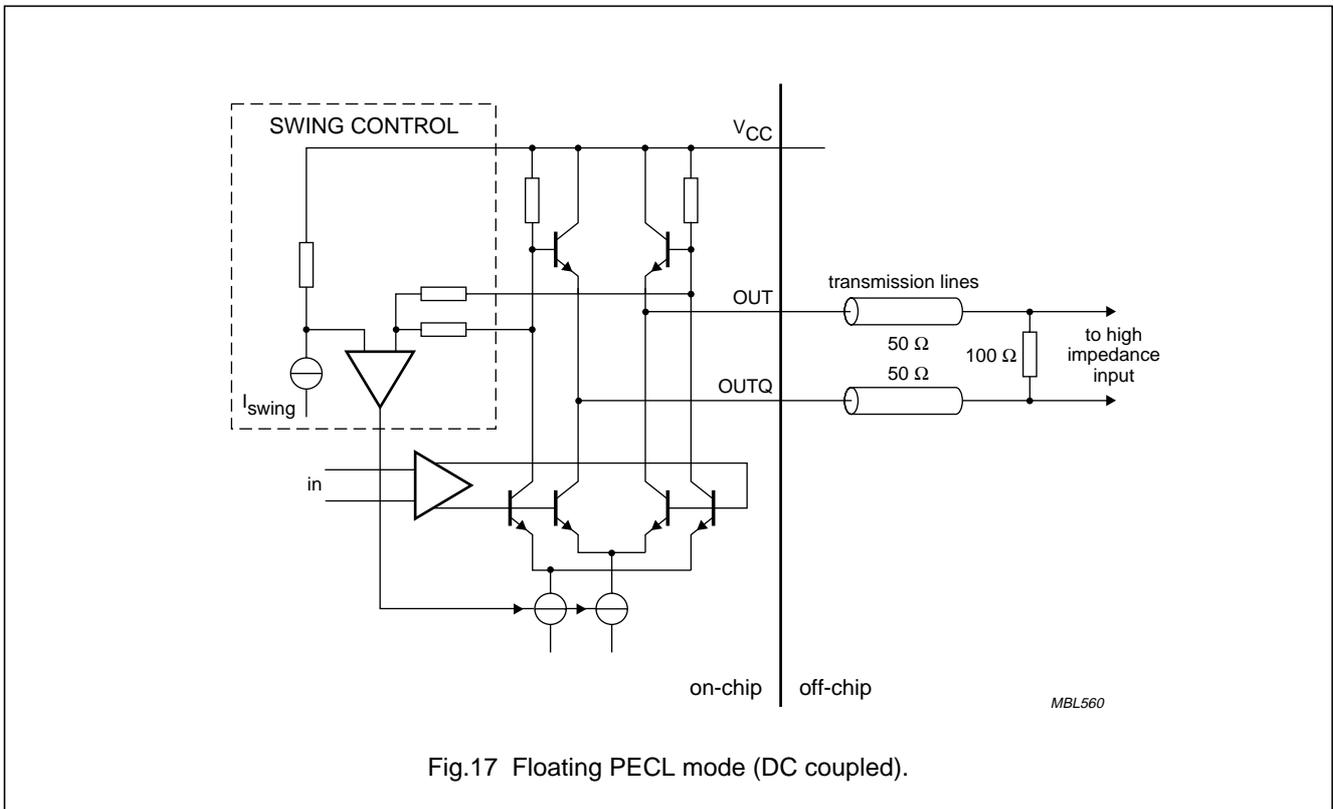
Fig.17 Floating PECL mode (DC coupled).
