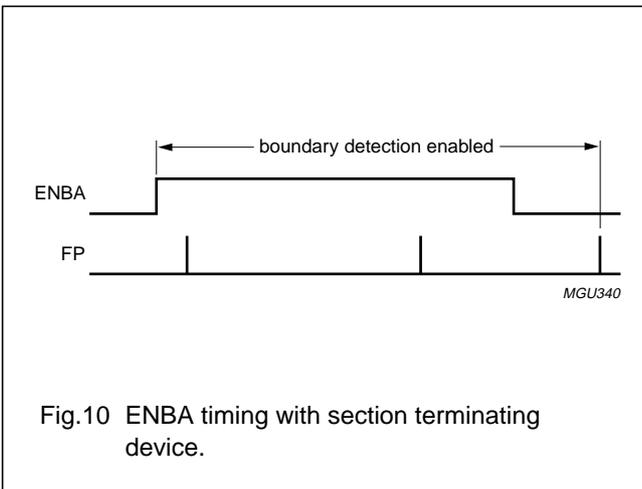
Fig.10 ENBA timing with section terminating device.
