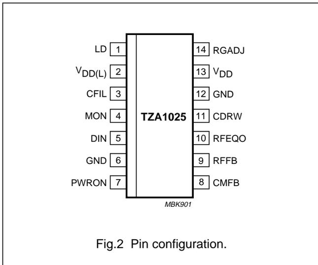
Fig.2 Pin configuration.
