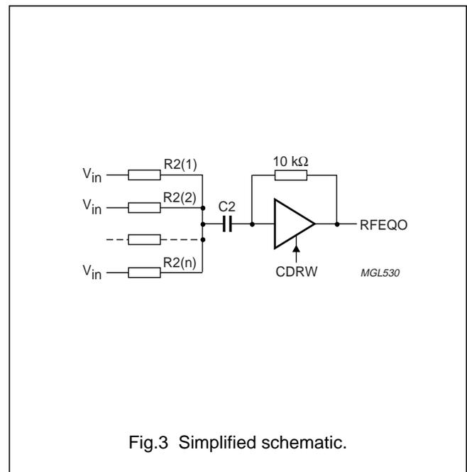
Fig.3 Simplified schematic.
