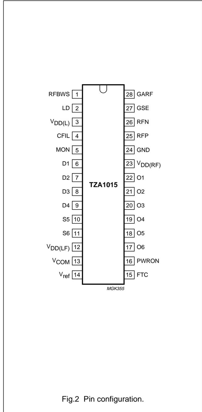
Fig.2 Pin configuration.
