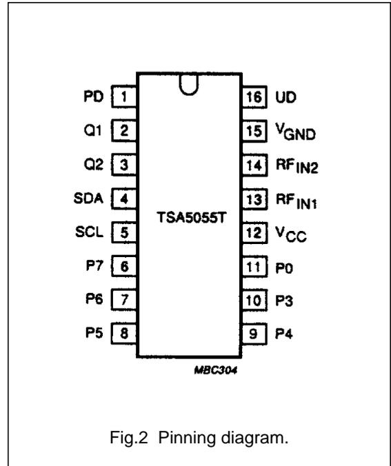
Fig.2 Pinning diagram.
