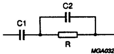
Fig.6 Loop filter.
