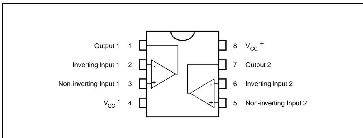
**SCHEMATIC DIAGRAM** (for 1/2 TS3V393)
