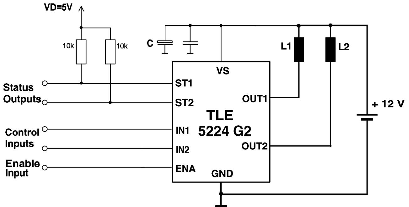
The blocking capacitor C is recommended to avoid critical negative voltage spikes on  $V_s$  in case of battery interruption during OFF-commutation.
