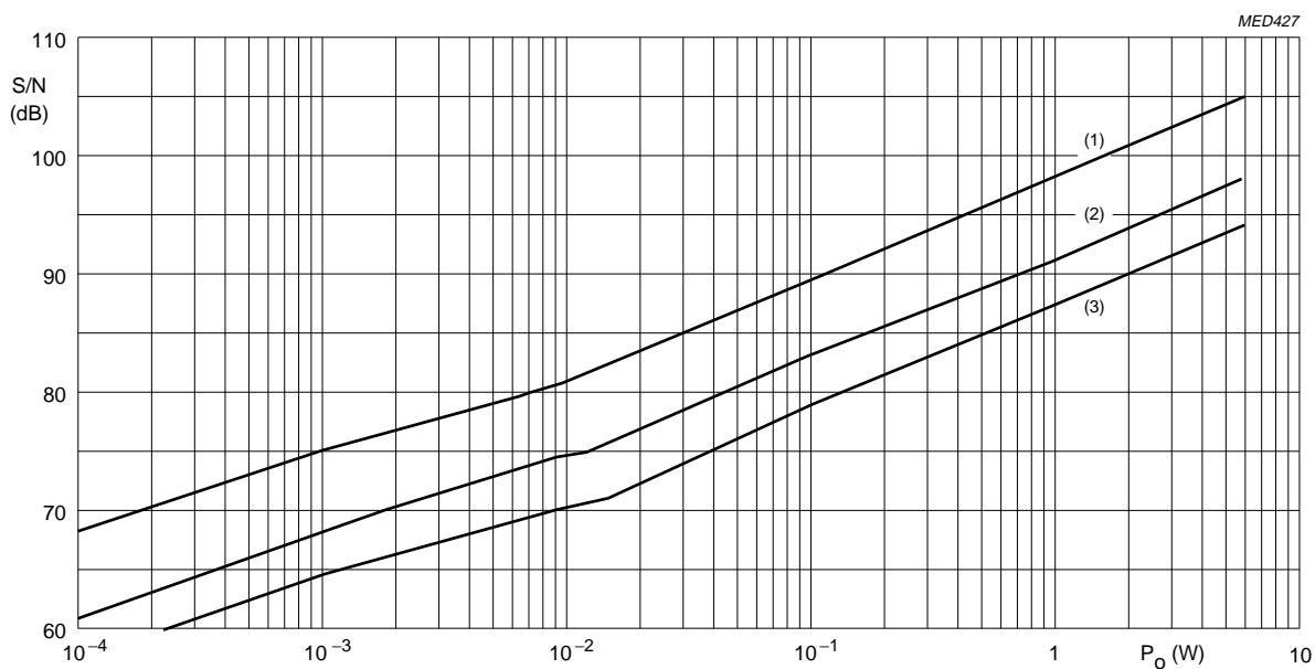
Fig.7 Signal-to-noise ratio;  $V_i = 2$  V;  $P_{\max} = 6$  W.
