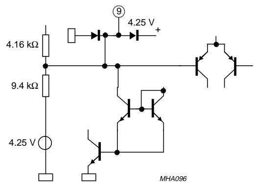
Fig.20 Pins 9 and 32: bass control capacitor inputs.
