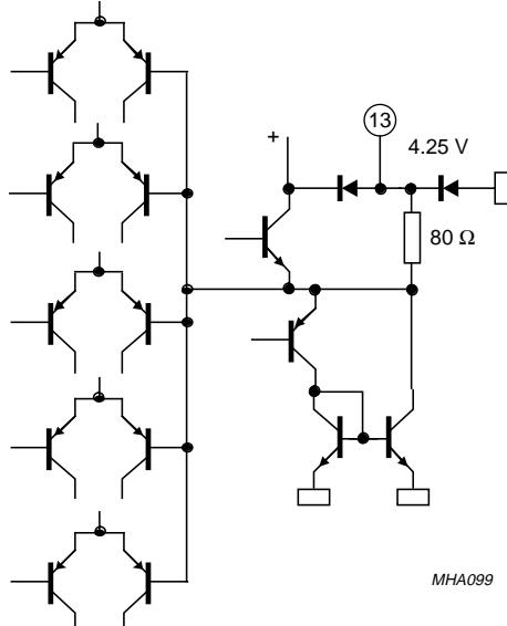
Fig.23 Pins 13 and 28: output source selector.
