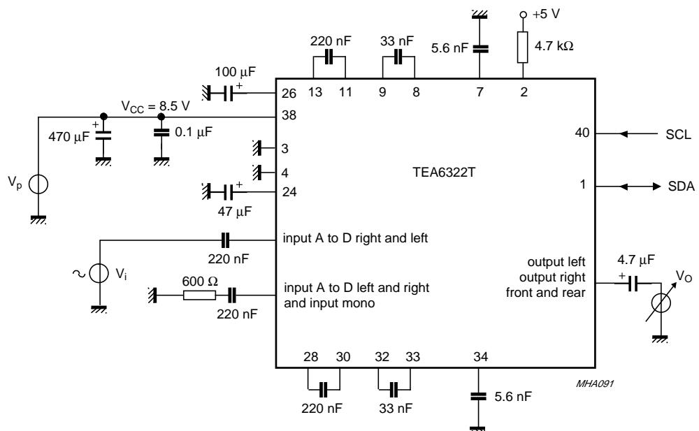
Fig.14 Test circuit for channel separation ( $\alpha_{cs}$ ).
