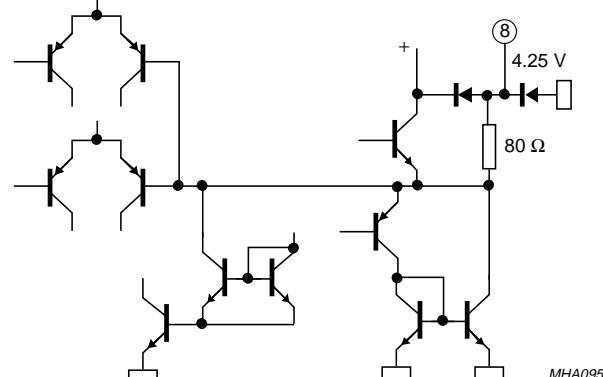
Fig.19 Pins 8 and 33: bass control capacitor outputs.
