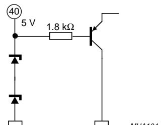
Fig.28 Pin 40: SCL (I<sup>2</sup>C-bus clock).
