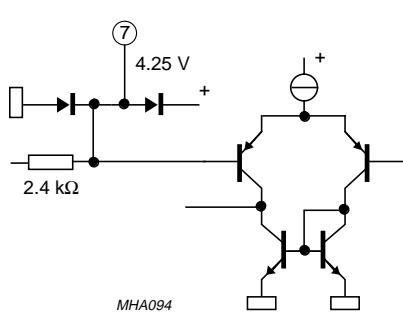
Fig.18 Pins 7 and 34: treble control capacitors.
