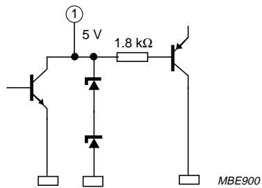
Fig.16 Pin 1: SDA (I<sup>2</sup>C-bus data).
