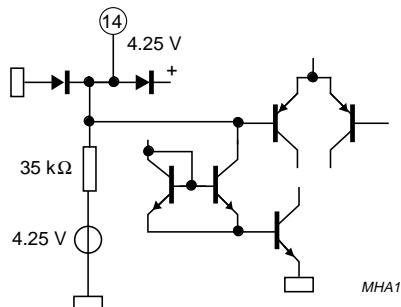
Fig.24 Pins 14, 16 to 18, 20, 21, 23, 25, 27: inputs.
