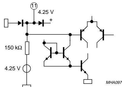
Fig.21 Pins 11 and 30: input volume 1, control part.
