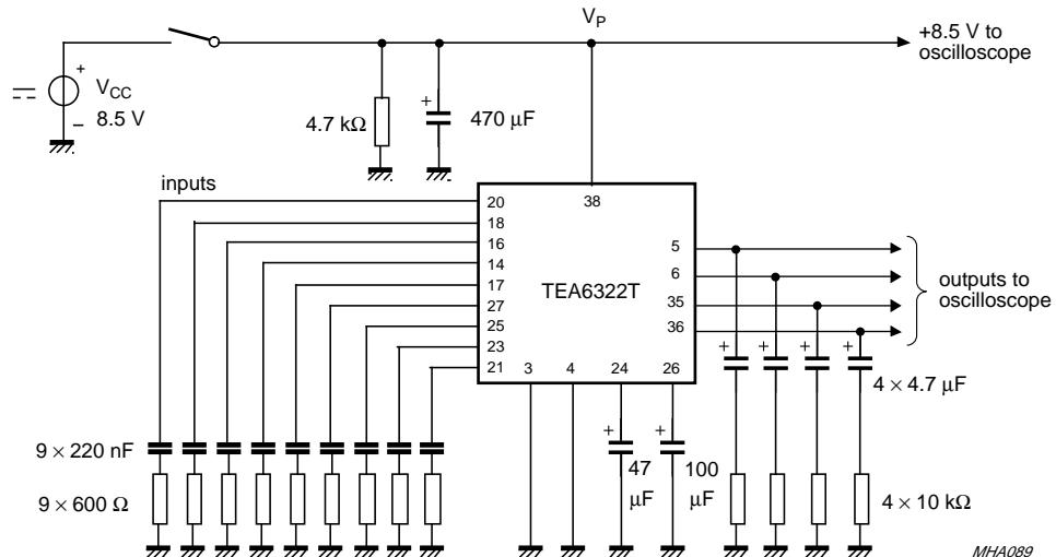
Fig.11 Turn-on/off power supply circuit diagram.
