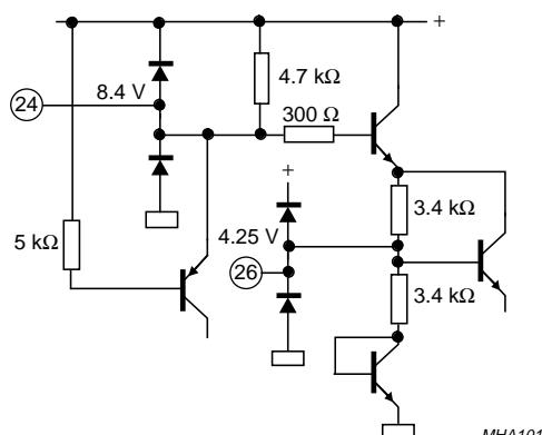
Fig.26 Pin 24: filtering for supply; pin 26: reference voltage.
