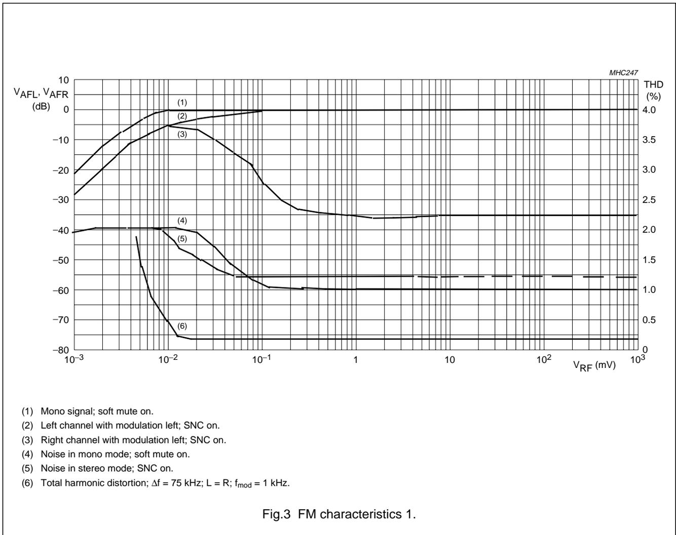
Low-power FM stereo radio for handheld applications
