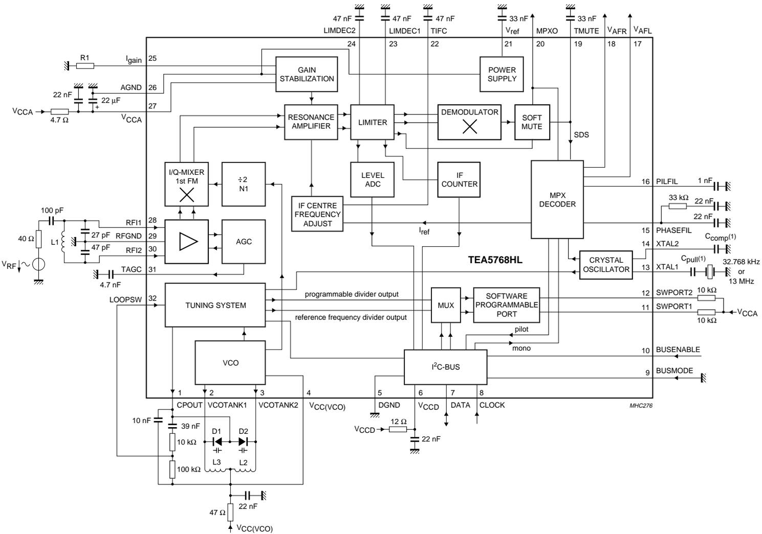
(1) C<sub>comp</sub> and C<sub>pull</sub> data depends on crystal specification.
