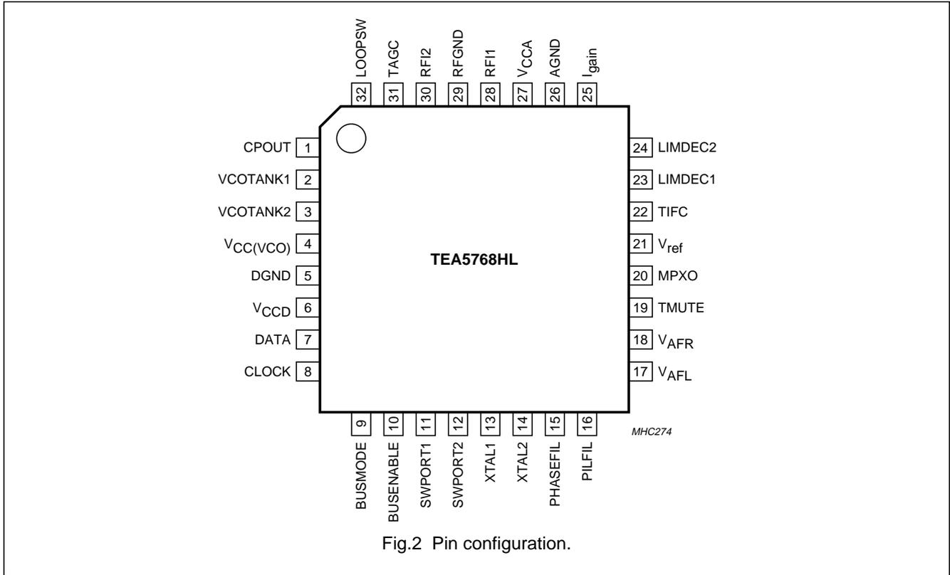
Fig.2 Pin configuration.
