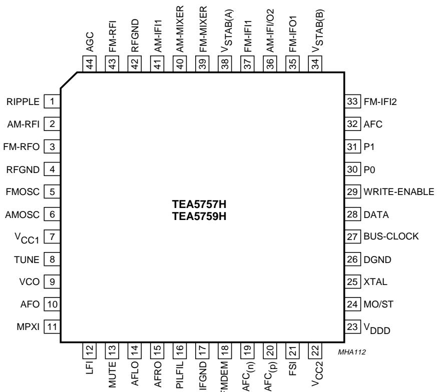
Fig.2 Pin configuration.
