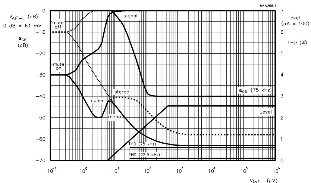
Fig.11 Typical FM audio voltage ( $V_{AF}$ ; signal), noise, THD (at  $\Delta f = 22.5$  kHz and  $\Delta f = 75$  kHz) and indicator current (level) as a function of RF input voltage ( $V_{in1}$ ;  $\Delta f = 22.5$  kHz). Curves are shown without mute (mono) and with mute (mono and stereo). Channel separation at  $\Delta f = 75$  kHz. Measured in test circuit Fig.7 with  $V_P = 3.0$  V.
