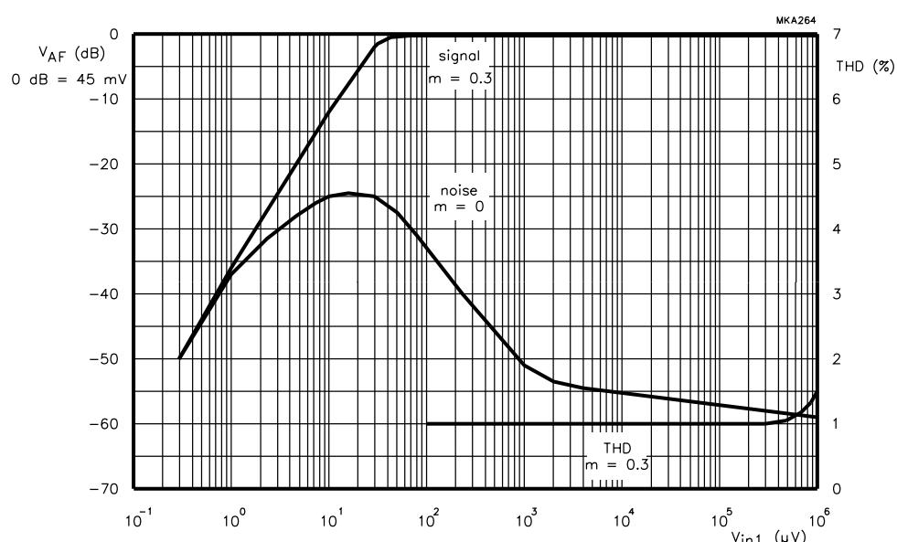
Fig.9 Typical AM audio voltage ( $V_{AF}$ ; signal at  $m = 0.3$ ), noise and THD as a function of RF input voltage ( $V_{in1}$ ;  $f_i = 1$  kHz). Measured in test circuit Fig.7 with  $V_P = 3.0$  V.
