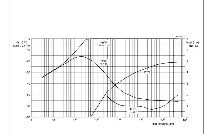
Fig.9 Typical AM audio output voltage ( $V_{AF}$ ; signal at m = 0.3), noise, THD (at m = 0.3) and indicator current (level) as a function of field-strength (f = 1 kHz). Measured at 1 MHz in application circuit of Fig.5 with  $V_P = 3 \text{ V}$ .
