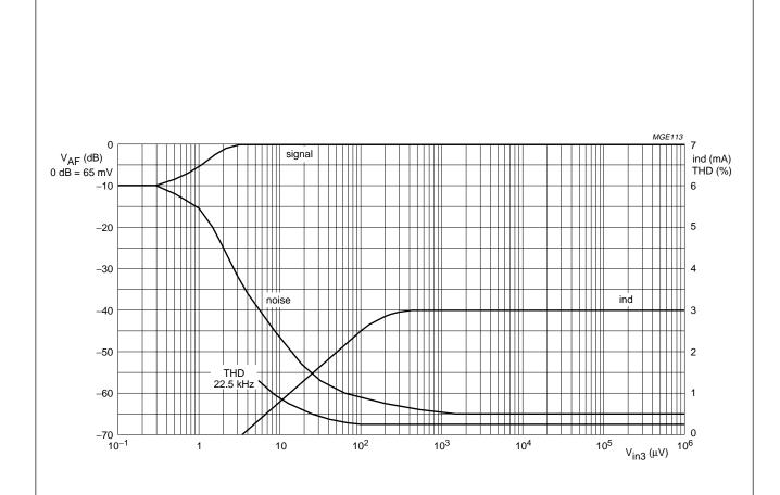
Fig.10 Typical FM audio output voltage ( $V_{AF}$ ; signal), noise, THD and indicator current (ind) as a function of RF input voltage ( $V_{in3}$ ;  $d_f = 22.5$  kHz). Measured in test circuit of Fig.4 at  $V_P = 3$  V.
