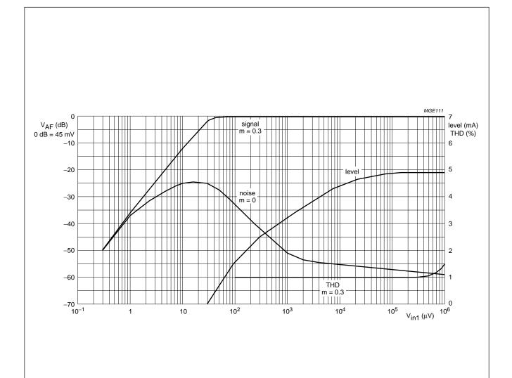
Fig.8 Typical AM audio output voltage ( $V_{AF}$ ; signal at m = 0.3), noise, THD (at m = 0.3) and indicator current (level) as a function of RF input voltage ( $V_{in1}$ ; f = 1 kHz). Measured in test circuit of Fig.4 with  $V_P = 3.0 \text{ V}$ .
