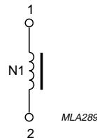
Fig.7 FM-RF coil (L1). TOKO equivalent no. MC115.
