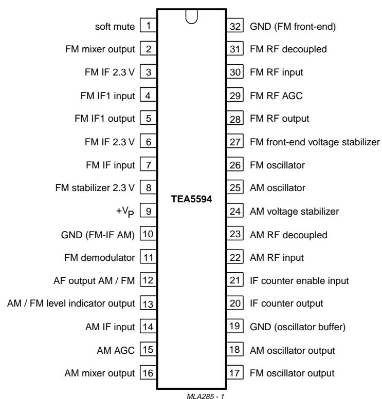
Fig.3 Pinning diagram.
