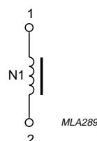
Fig.8 FM oscillator coil (L2). TOKO equivalent no. A294SNS-1004NK.
