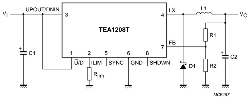
Fig.6 Complete application diagram for down conversion.
