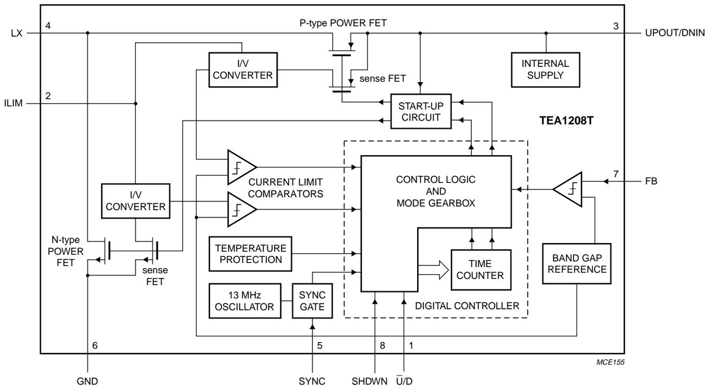
Fig.1 Block diagram.
