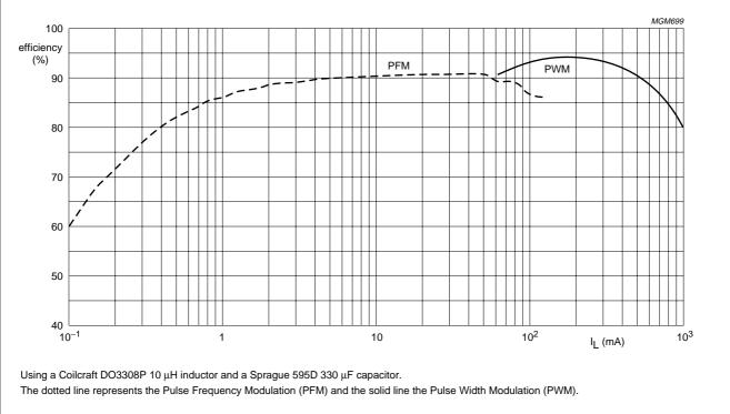
Fig.6 Efficiency as a function of load current  $I_L$  (2.4 to 3.3 V).
