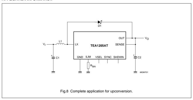
A typical component choice for an upconverter from 3 NiCd cells or one Li-ion cell to 5.0 V in a GSM handset (peak power 7.5 W, peak current 2.7 A) is (see Fig.8):
