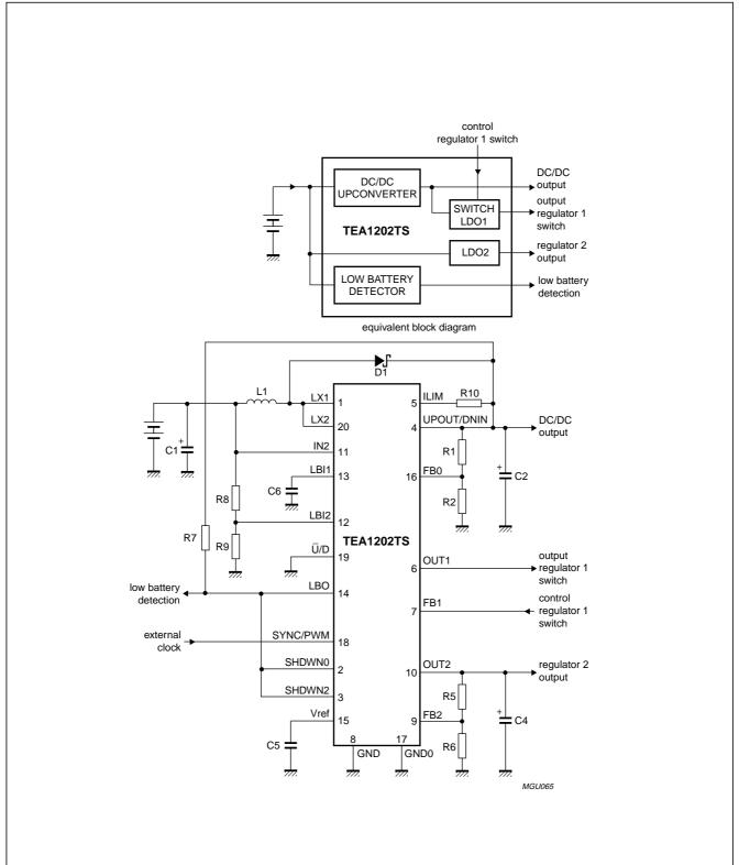
Fig.7 Application in two-cell NiCd or NiMH battery powered equipment with autonomous shut-down at low battery voltage and using LDO1 as a switch.
