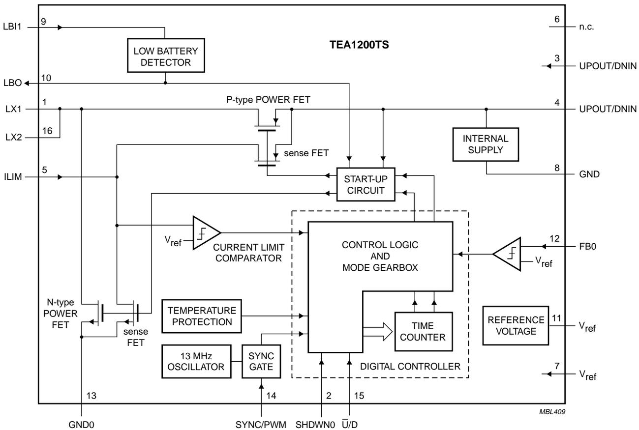
Fig.1 Block diagram.
