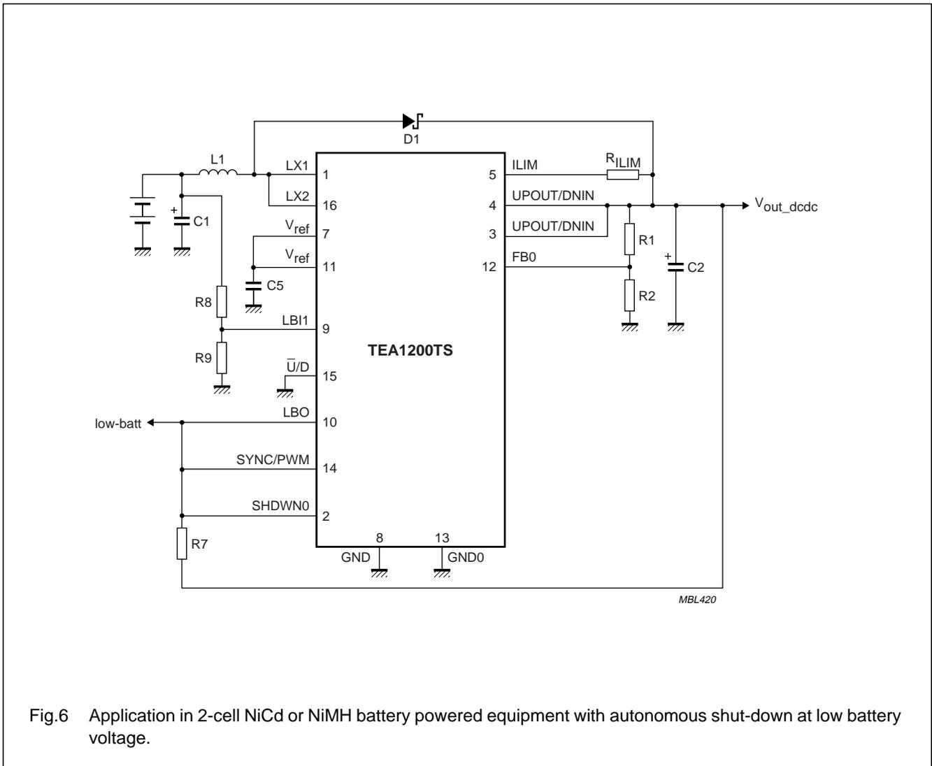
Fig.6 Application in 2-cell NiCd or NiMH battery powered equipment with autonomous shut-down at low battery voltage.
