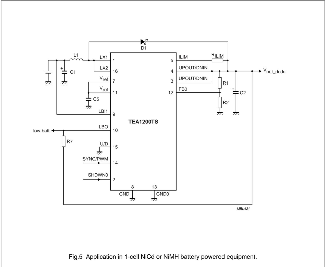
Fig.5 Application in 1-cell NiCd or NiMH battery powered equipment.
