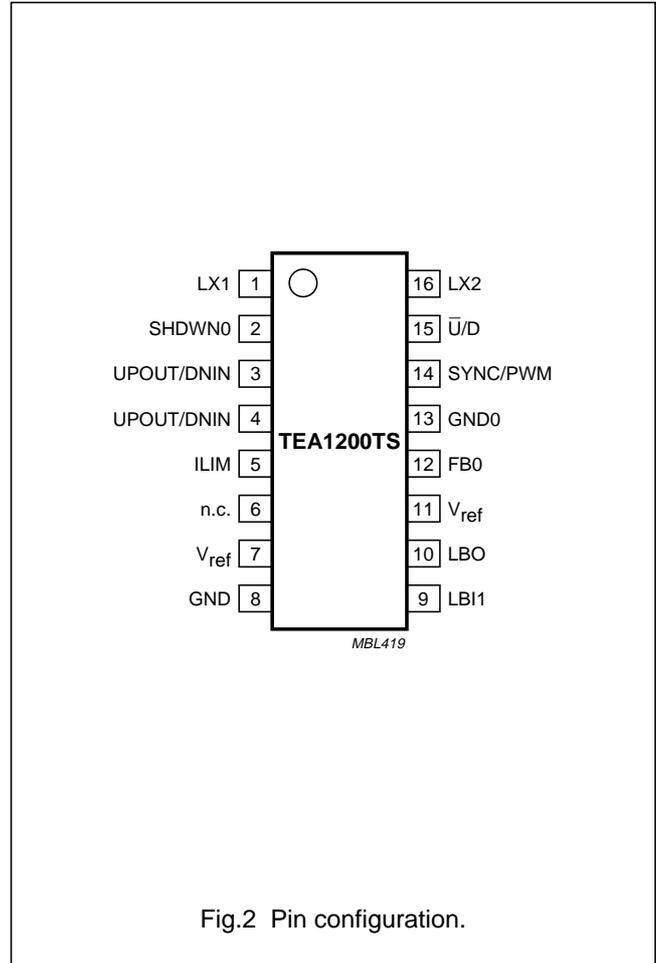
Fig.2 Pin configuration.
