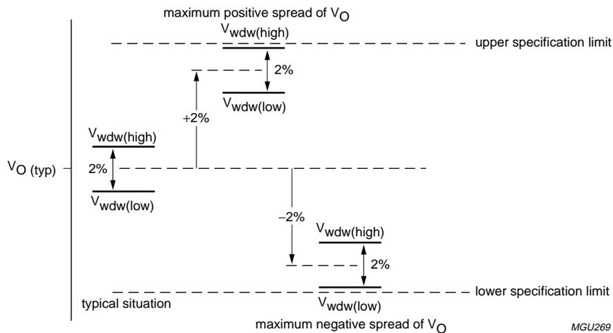
Fig.4 Output voltage window spread.
