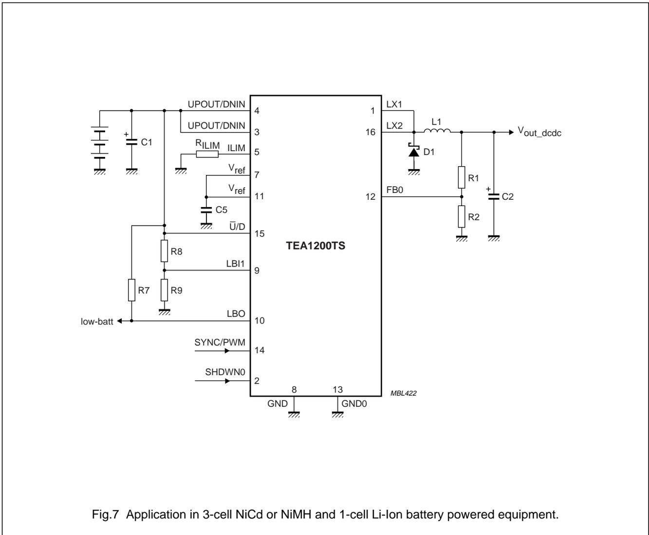
Fig.7 Application in 3-cell NiCd or NiMH and 1-cell Li-Ion battery powered equipment.
