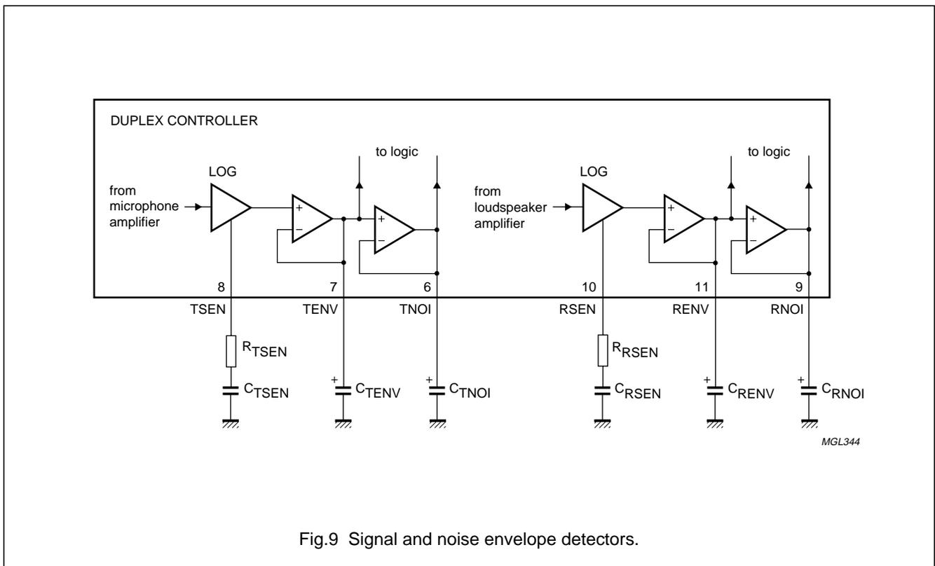
Fig.9 Signal and noise envelope detectors.
