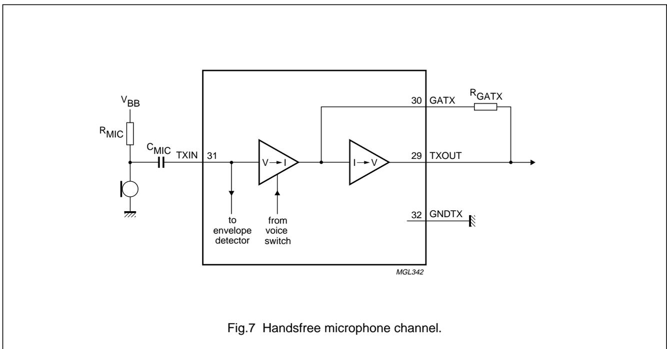
Fig.7 Handsfree microphone channel.
