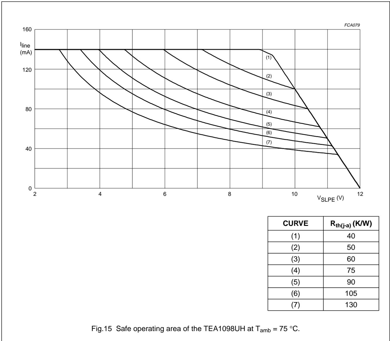
Fig.15 Safe operating area of the TEA1098UH at  $T_{amb} = 75\text{ °C}$ .
