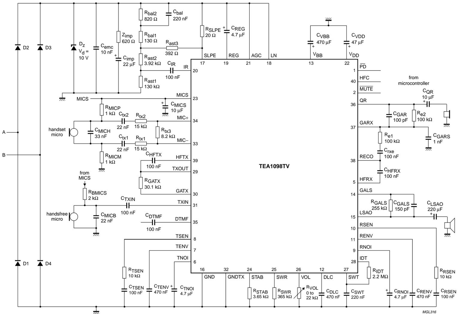
Fig.17 Basic application diagram.
