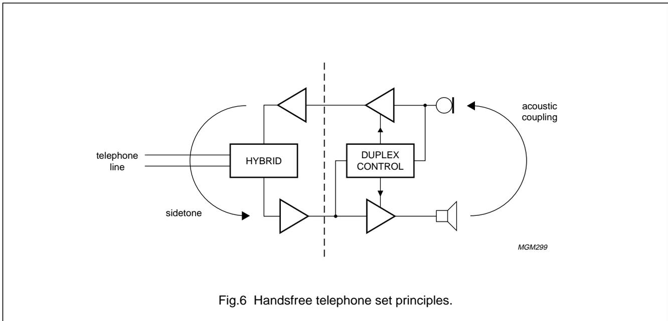
Fig.6 Handsfree telephone set principles.
