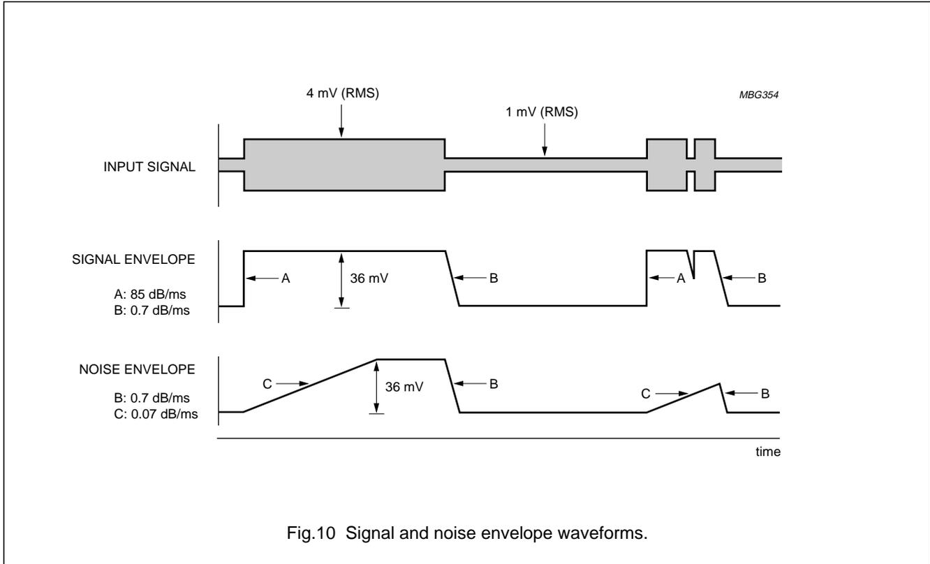
Fig.10 Signal and noise envelope waveforms.
