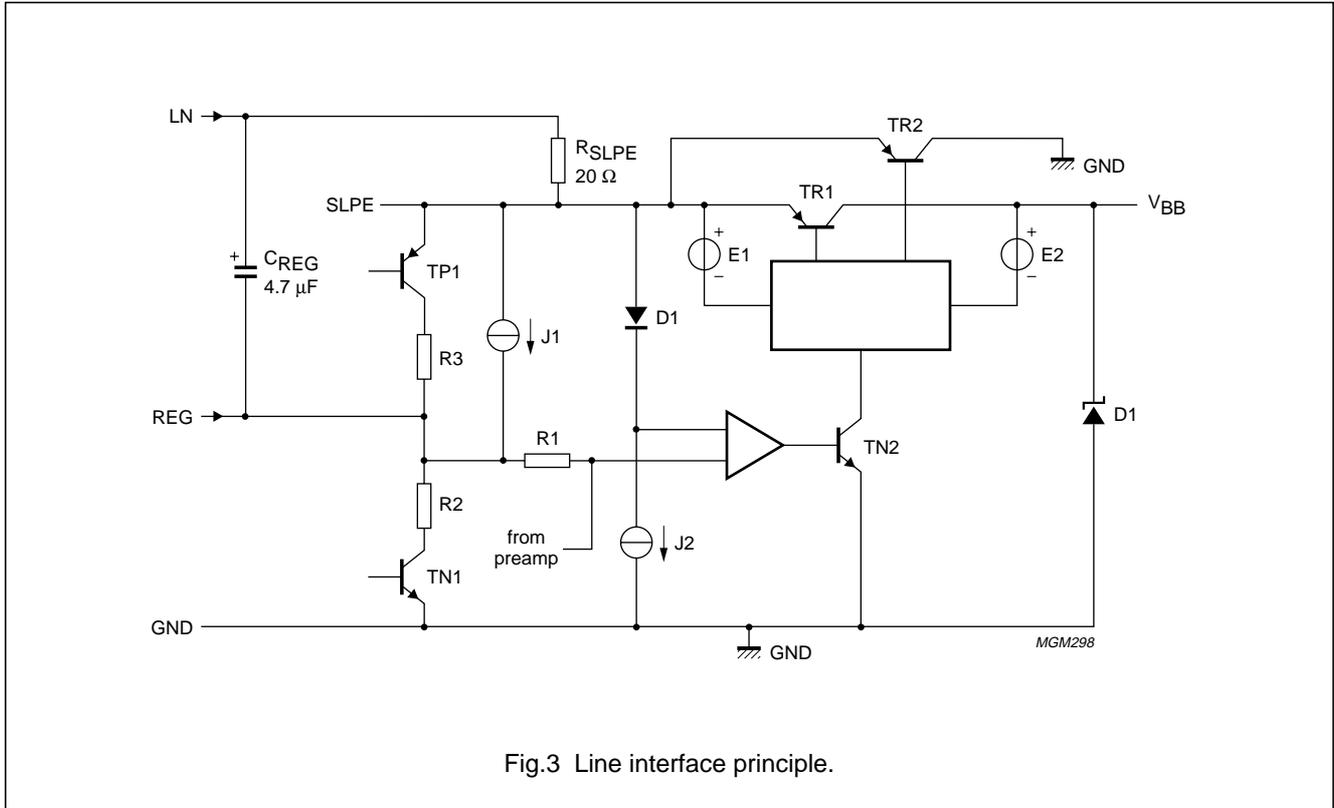
Fig.3 Line interface principle.
