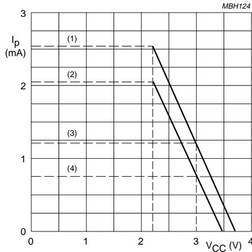
Curve (1) is valid when the receiving amplifier is not driven or when MUTE = HIGH. Curve (2) is valid when MUTE = LOW and the receiving amplifier is driven;  $V_{o(rms)} = 150\text{ mV}$ ;  $R_L = 150\ \Omega$  asymmetrical.
