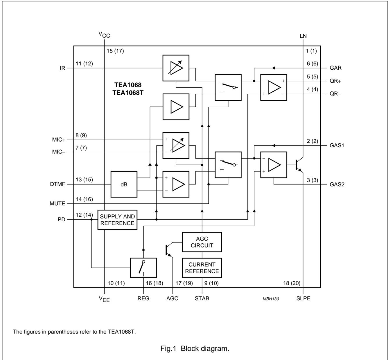
Versatile telephone transmission circuit
