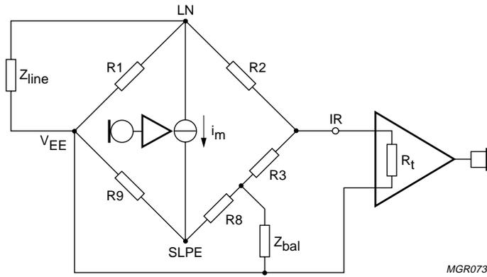
Fig.18 Equivalent circuit of TEA1060 family anti-side-tone bridge.
