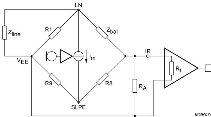
Fig.19 Equivalent circuit of an anti-sidetone network in the Wheatstone bridge configuration.
