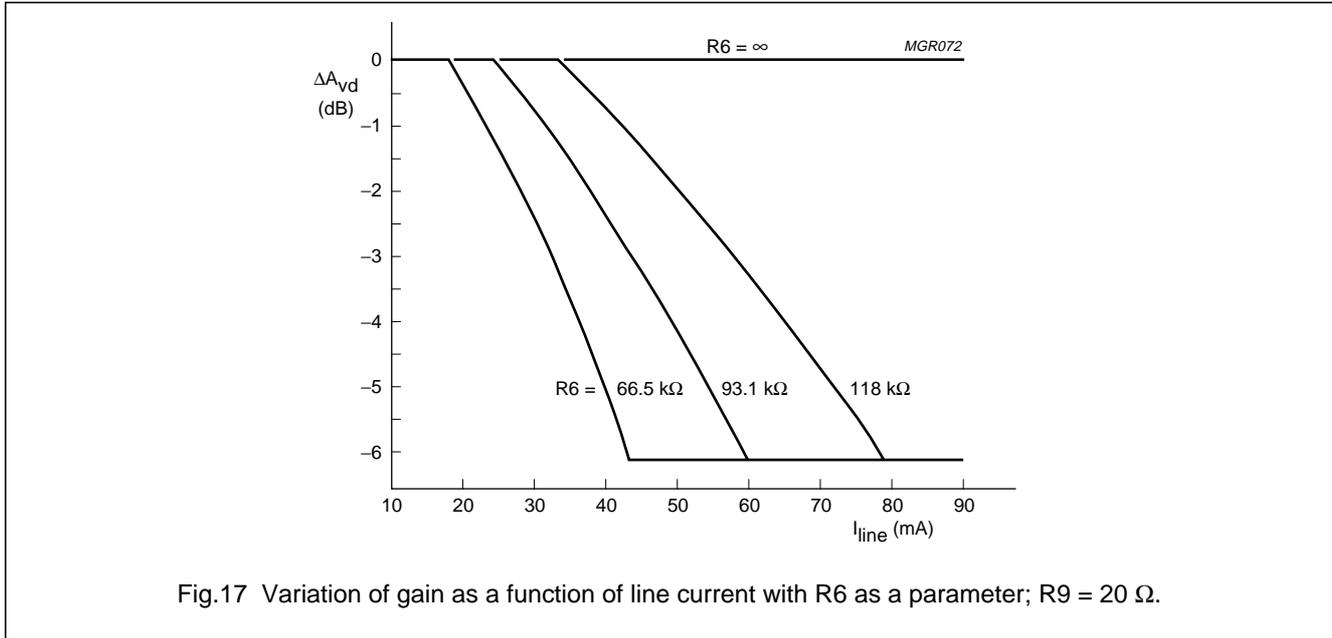
Fig.17 Variation of gain as a function of line current with R6 as a parameter; R9 = 20 Ω.
