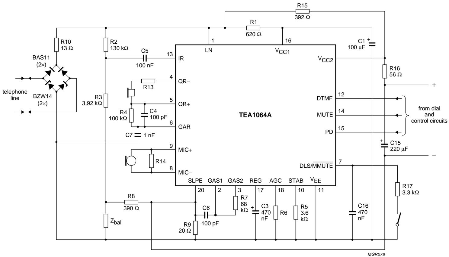
Fig.24 Basic application of the TEA1064A with stabilized supply for peripherals, shown here with a piezo-electric earpiece and DTMF dialling. The diode bridge and R10 limit the current into, and the voltage across, the circuit during line transients. A different protection arrangement is required for pulse dialling or register recall.
