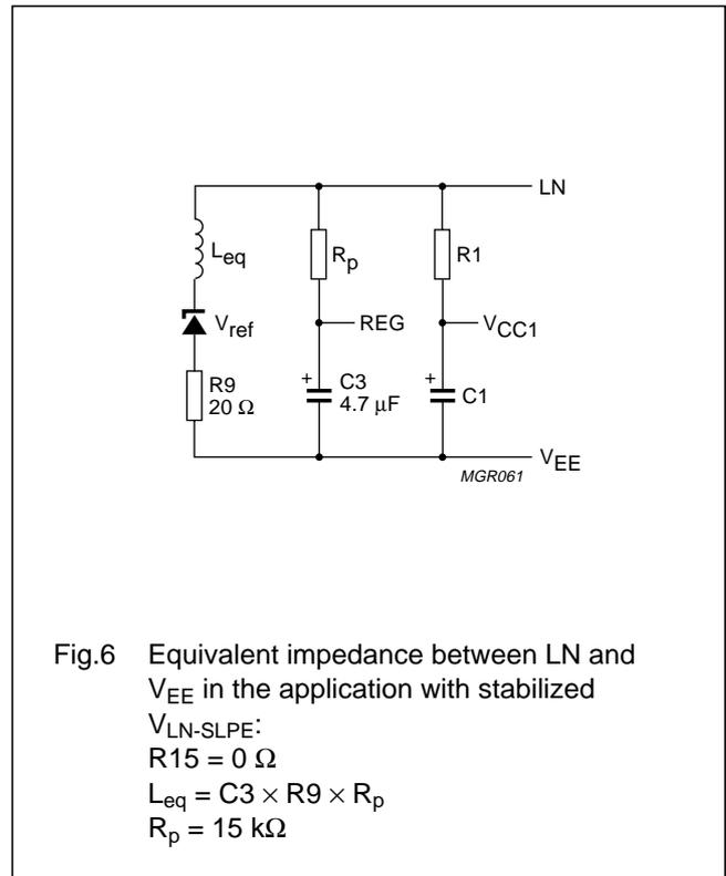
Fig.6 Equivalent impedance between LN and  $V_{EE}$  in the application with stabilized  $V_{LN-SLPE}$ :
