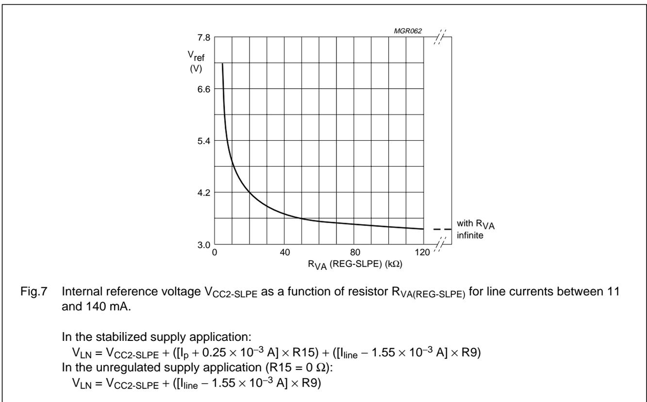
Fig.7 Internal reference voltage  $V_{CC2-SLPE}$  as a function of resistor  $R_{VA(REG-SLPE)}$  for line currents between 11 and 140 mA.
