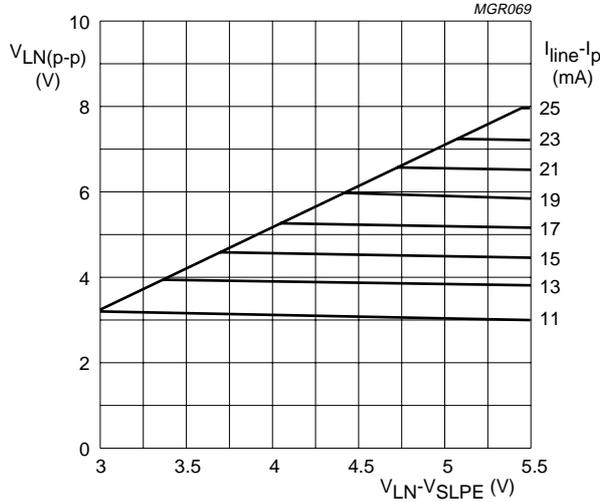
Fig.14 Maximum output swing on line as a function of the DC voltage drop  $V_{LN}-V_{SLPE}$  with  $I_{line} - I_p$  as a parameter:  $R_{15} = 392 \Omega$ ;  $R_{16} = 56 \Omega$ ; or  $R_{15} = 0 \Omega$  and  $R_{16} = 392 + 56 = 448 \Omega$ .
