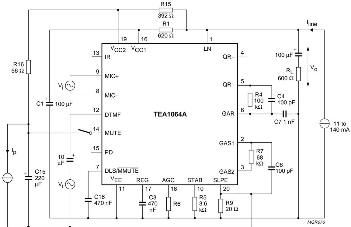
For measuring the gain from MIC+ and MIC- the MUTE input should be LOW or open-circuit; for measuring the DTMF input, the MUTE input should be HIGH. Inputs not being tested should be open-circuit.
