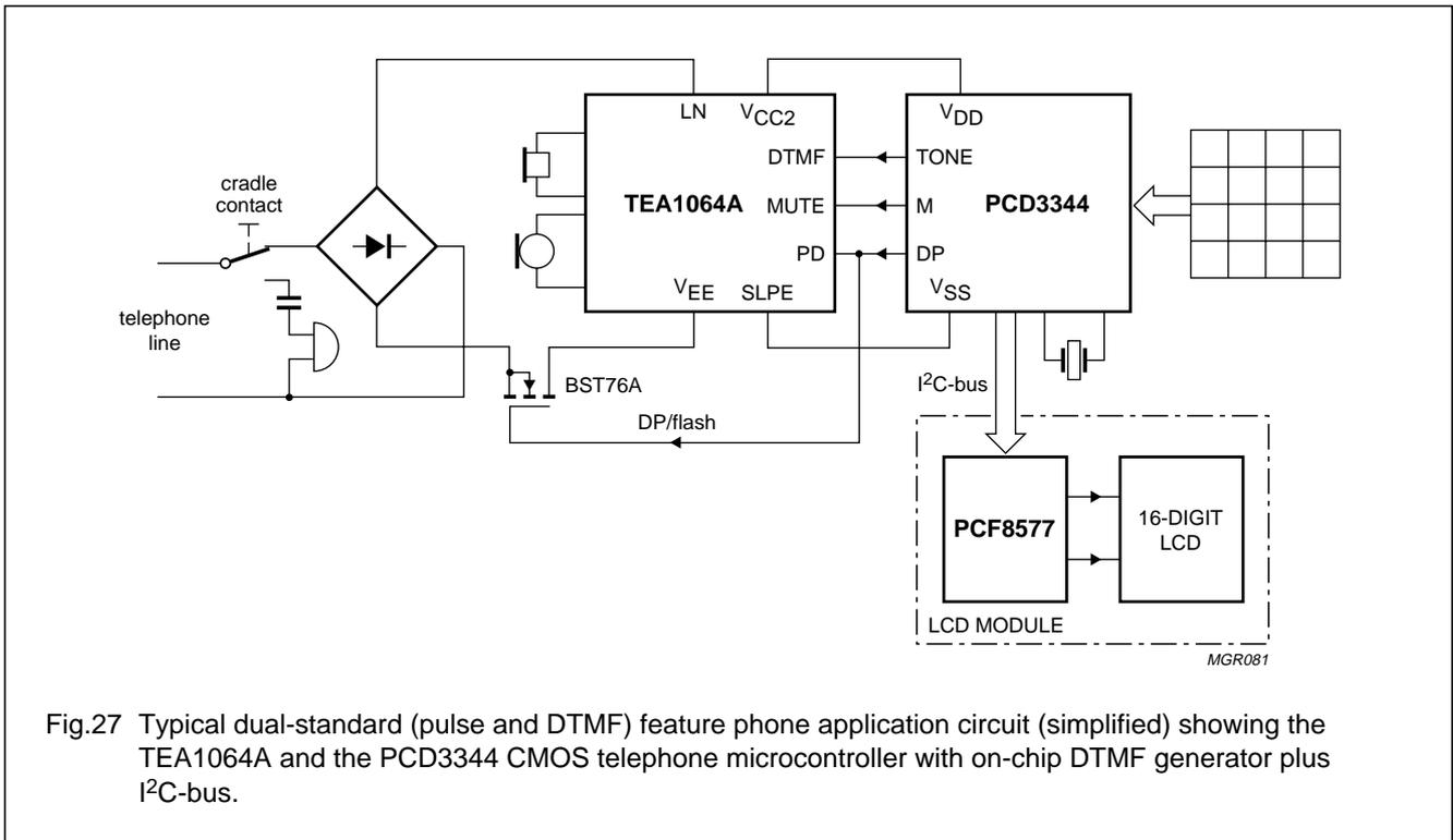
Fig.27 Typical dual-standard (pulse and DTMF) feature phone application circuit (simplified) showing the TEA1064A and the PCD3344 CMOS telephone microcontroller with on-chip DTMF generator plus I<sup>2</sup>C-bus.
