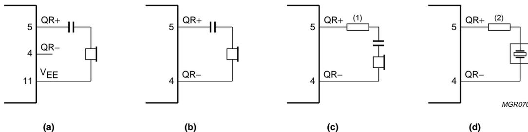
Fig.15 Alternative receiver arrangements: a) dynamic earpiece with an impedance less than  $450 \Omega$ ; b) dynamic earpiece with an impedance more than  $450 \Omega$ ; c) magnetic earpiece with an impedance more than  $450 \Omega$ , resistor (1) may be connected to prevent distortion (inductive load); d) piezo-electric earpiece, resistor (2) is required to increase the phase margin (stability with capacitive load).
