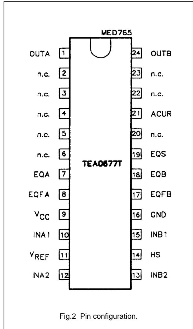
Fig.2 Pin configuration.
