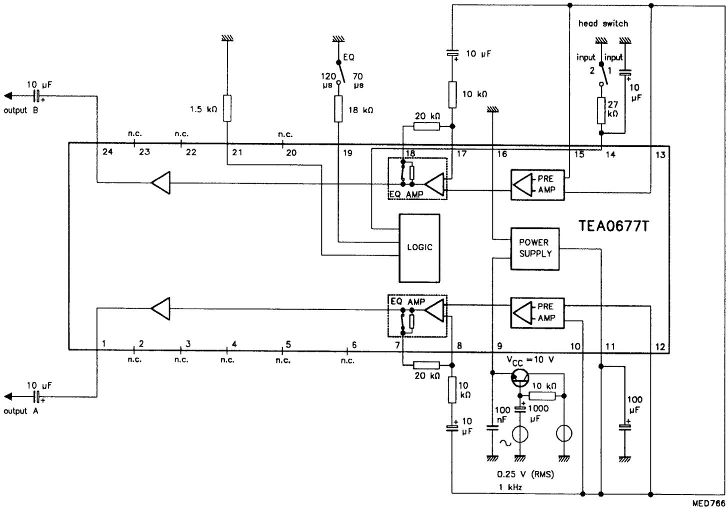
Fig.3 Test circuit for power supply ripple rejection.
