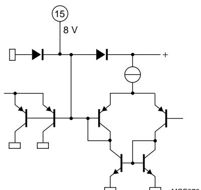
Fig.10 Pin 15: input equalizer switch.
