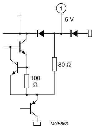
Fig.3 Pins 1 and 16: output channel.
