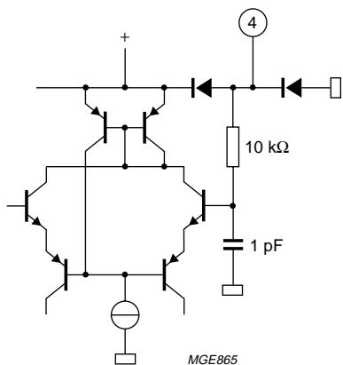
Fig.5 Pins 4 and 13: equalizer inputs.
