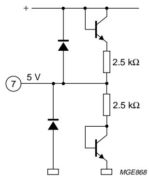
Fig.8 Pin 7: reference voltage.
