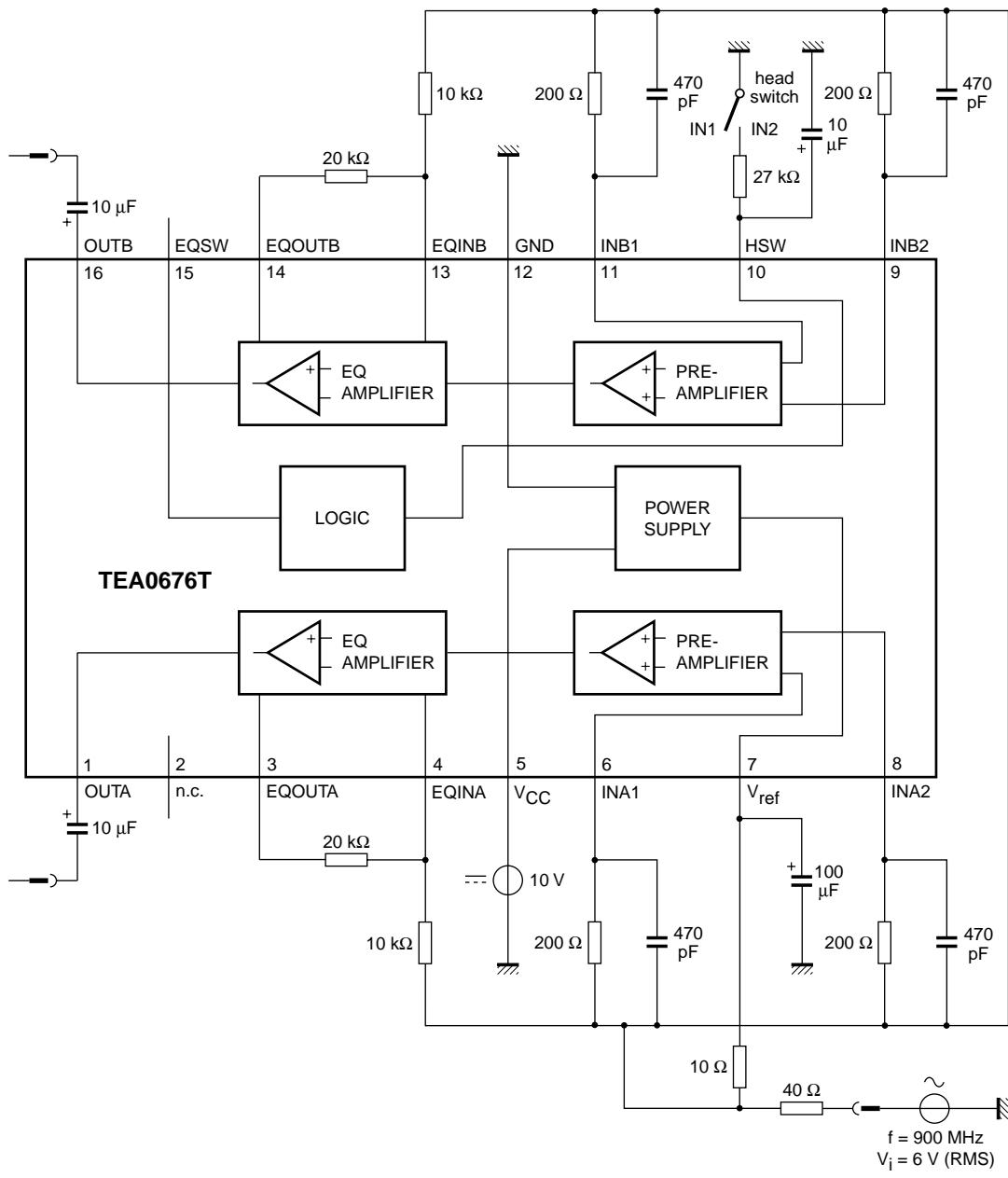
Fig.12 EMC test diagram.
