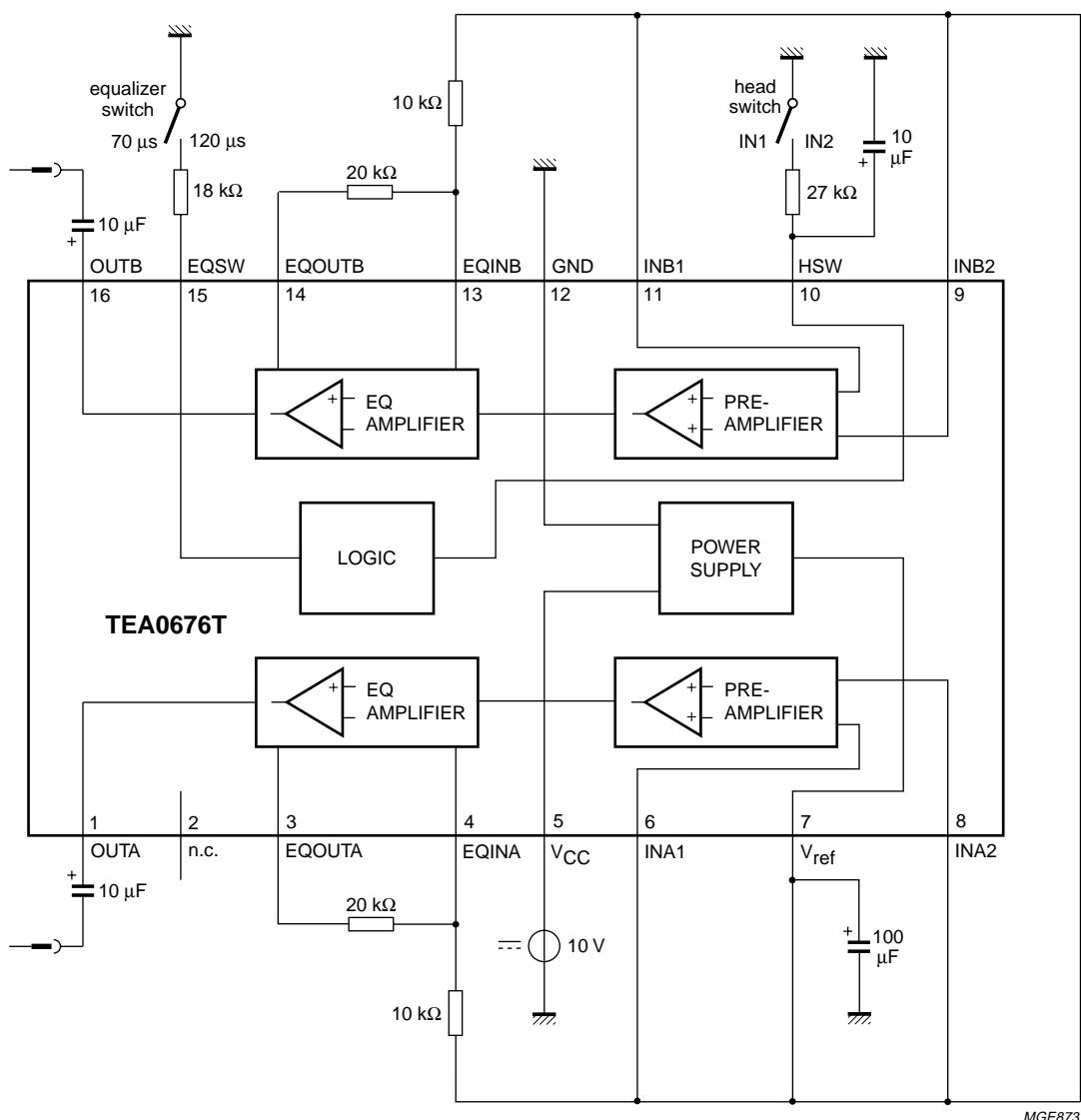
Fig.13 Noise test diagram.
