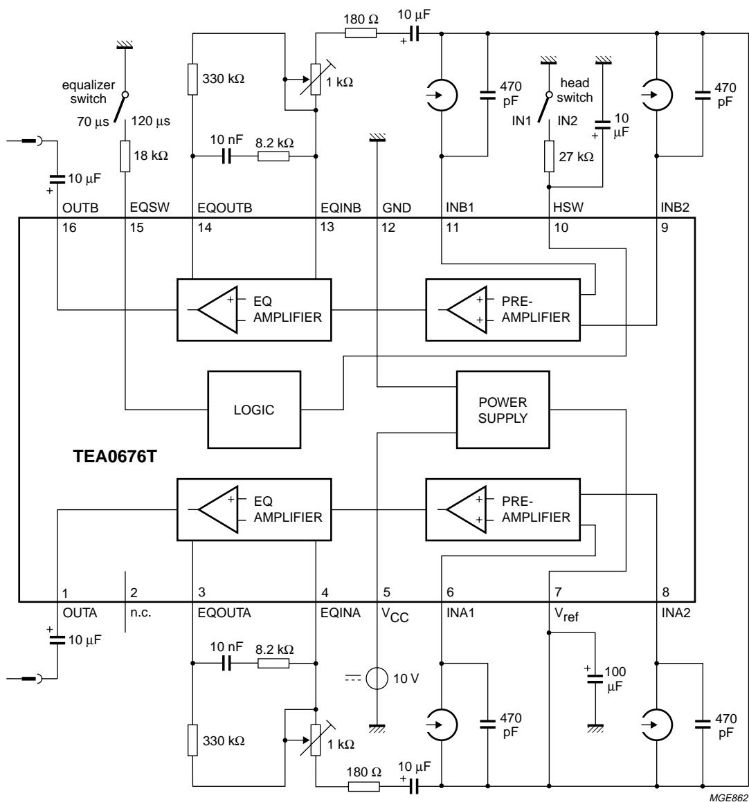
Fig.1 Block and application diagram.
