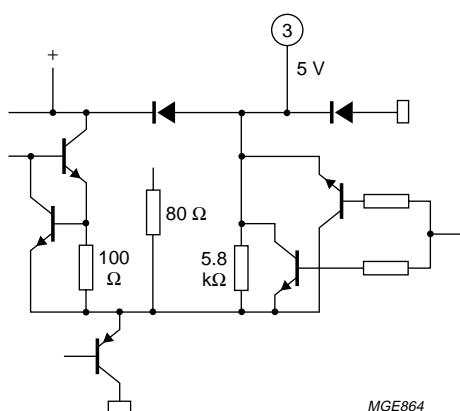
Fig.4 Pins 3 and 14: equalizer outputs.
