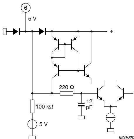
Fig.7 Pins 6, 8, 9, 11: input channel.
