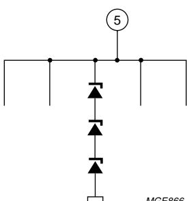
Fig.6 Pin 5: supply voltage.
