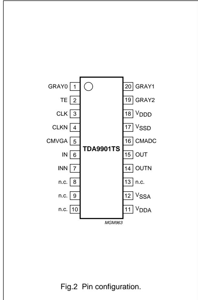
Fig.2 Pin configuration.
