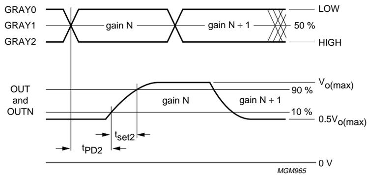
Fig.4 Transparent mode timing diagram with CLK HIGH.
