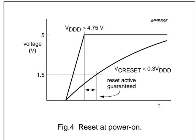
Fig.4 Reset at power-on.
