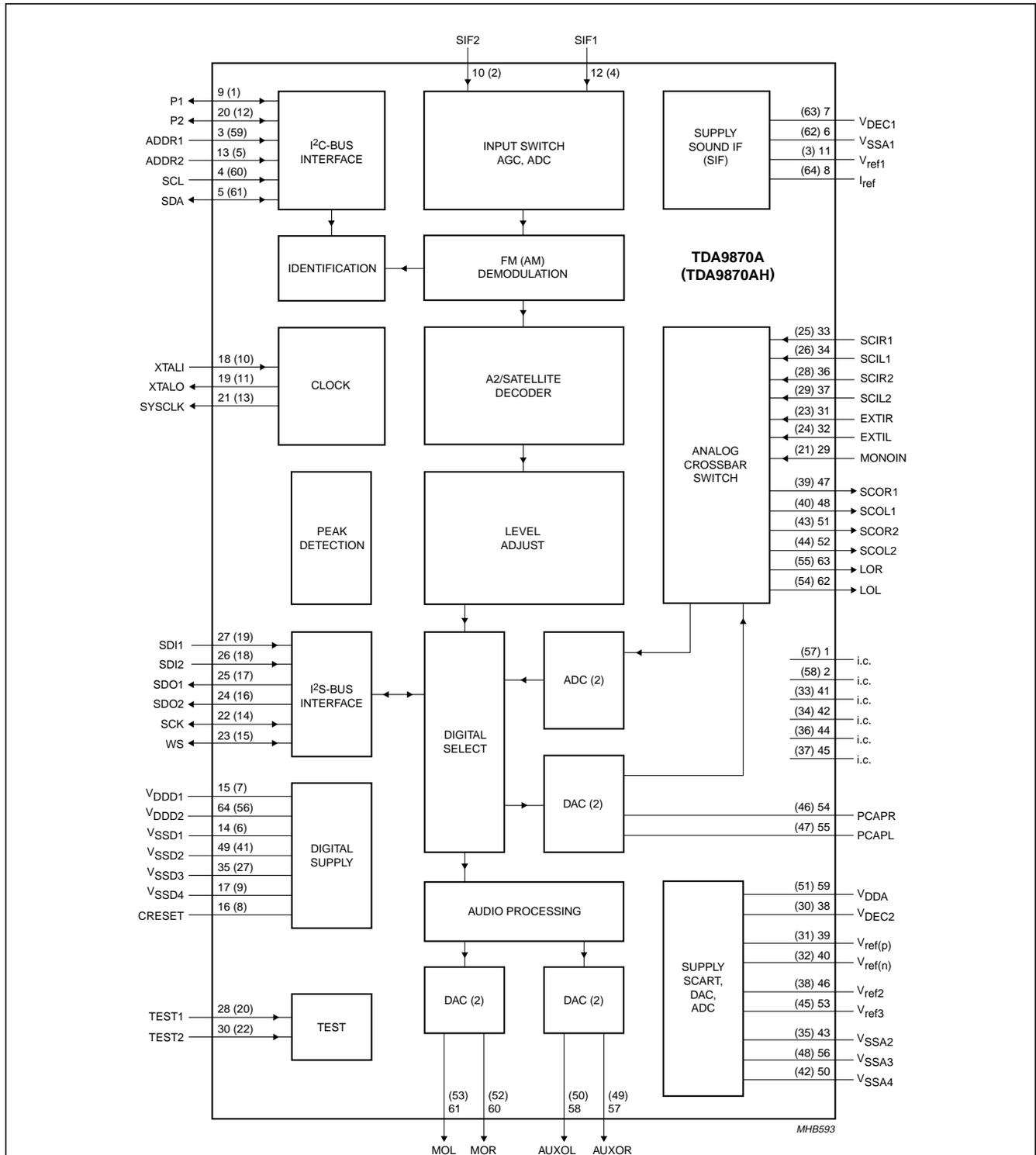
The pin numbers given in parenthesis refer to the TDA9870AH version.
