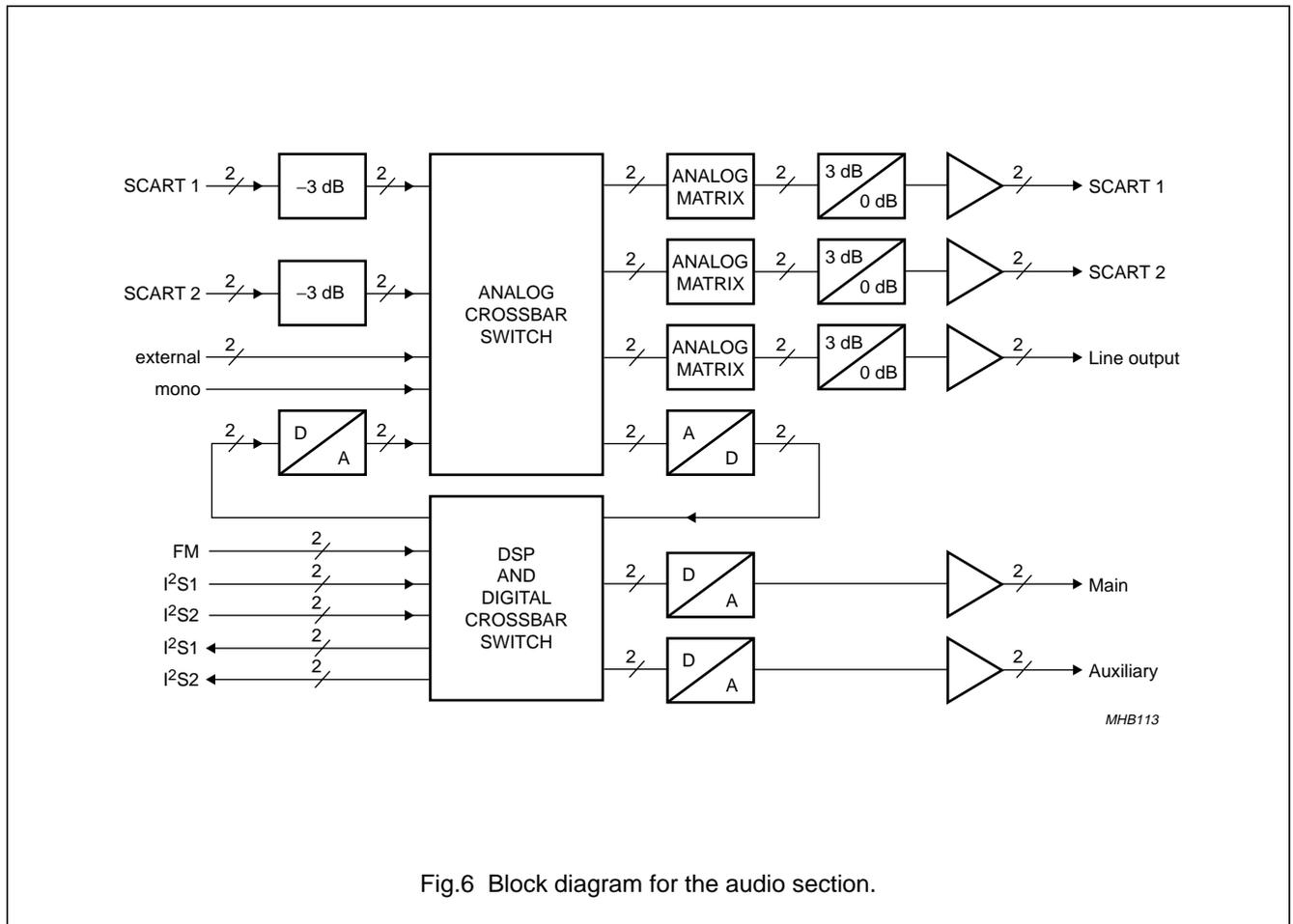
Fig.6 Block diagram for the audio section.
