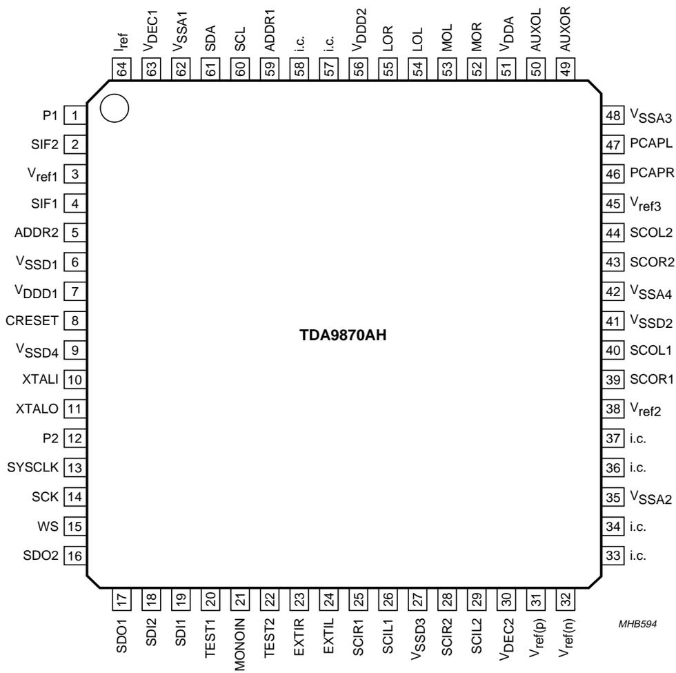
Fig.3 Pin configuration (TDA9870AH).
