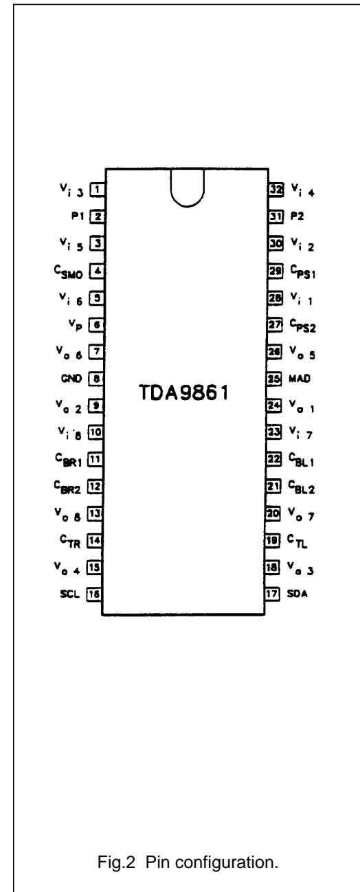
Fig.2 Pin configuration.
