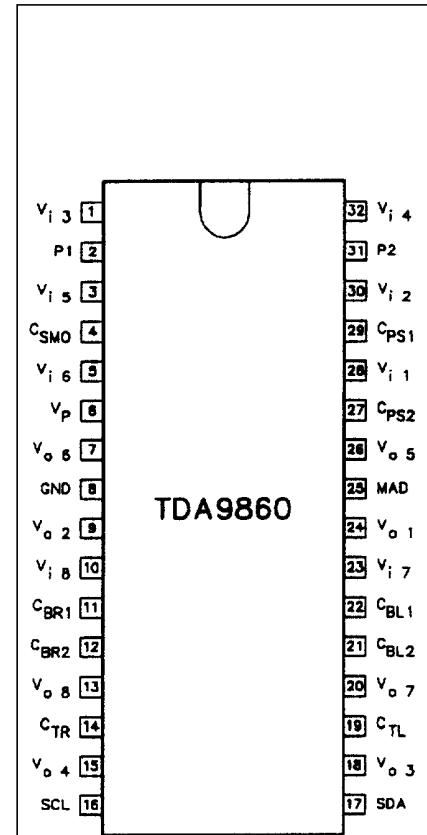
Fig.2 Pin configuration.
