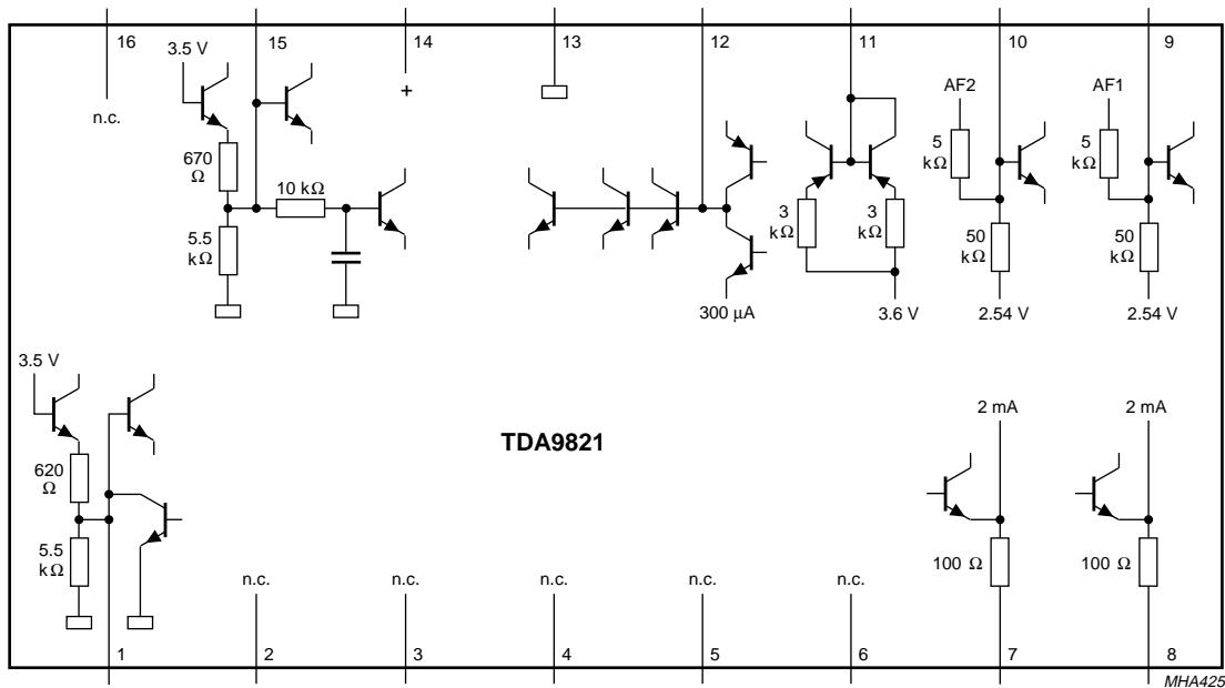
Fig.4 Internal circuitry.
