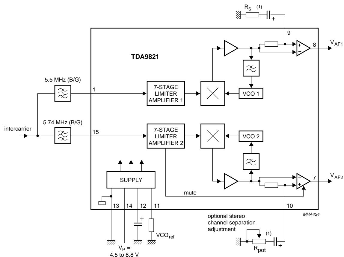
(1) Resistor and potentiometer between capacitor and earth are inserted if adjustment of stereo channel separation is required.
