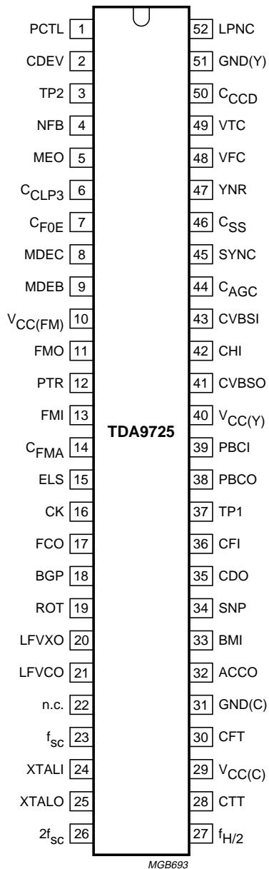
Fig.3 Pin configuration.
