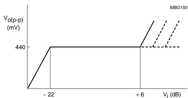
0 dB is equivalent to 110 mv (p-p) at pin 30.
