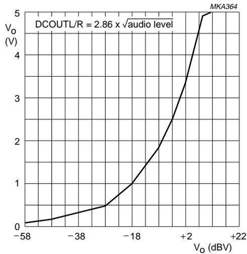
Fig.7 VU meter output voltage at DCOUTL and DCOUTR (pins 23 and 24) as a function of audio signal level.
