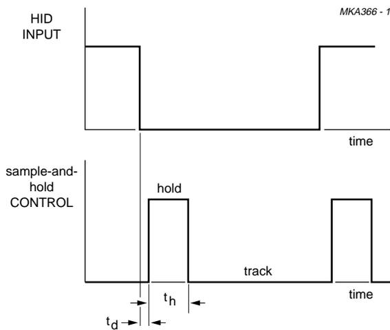
Fig.9 Sample-and-hold timing waveforms.
