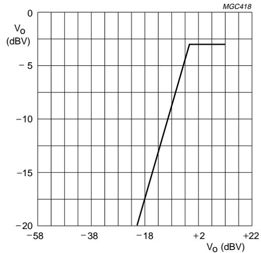
Fig.8 RF converter output voltage at RFCOUT (pin 18) as a function of line output signal level at LINEL and LINER (pins 21 and 22).
