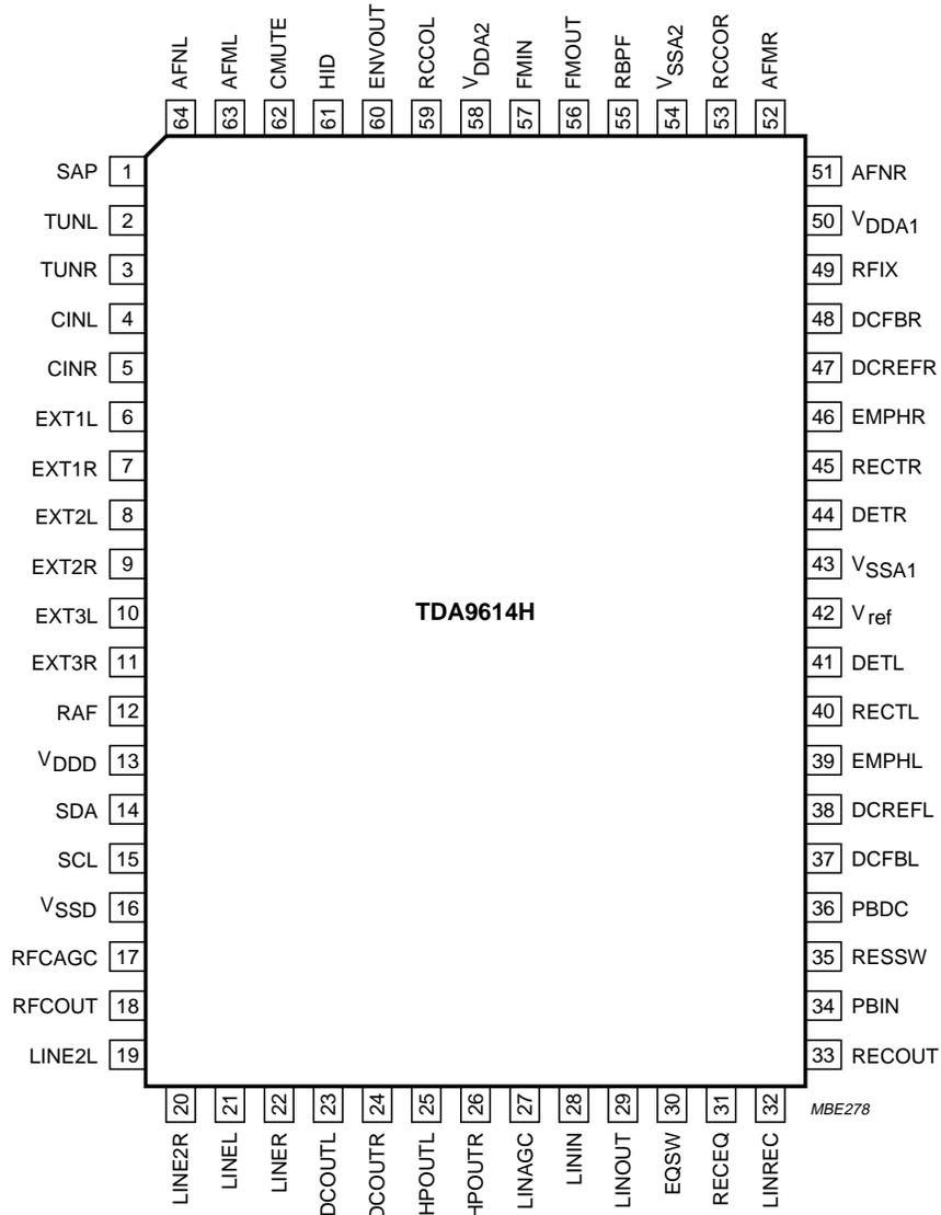
Fig.2 Pin configuration.
