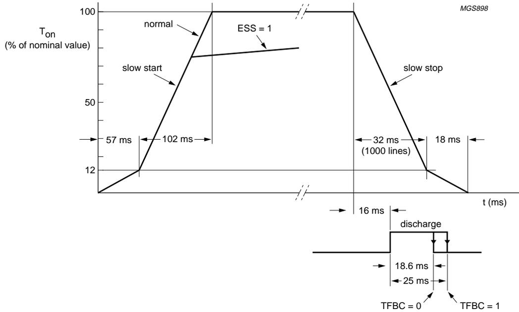
Fig.15 Slow start behaviour of horizontal output, and slow stop behaviour and timing of picture tube discharge pulse when IC is switched to standby via I<sup>2</sup>C-bus.
