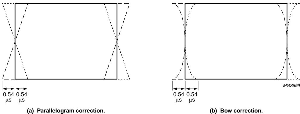
Fig.16 Horizontal parallelogram and bow correction (figures for 1f<sub>H</sub> mode).
