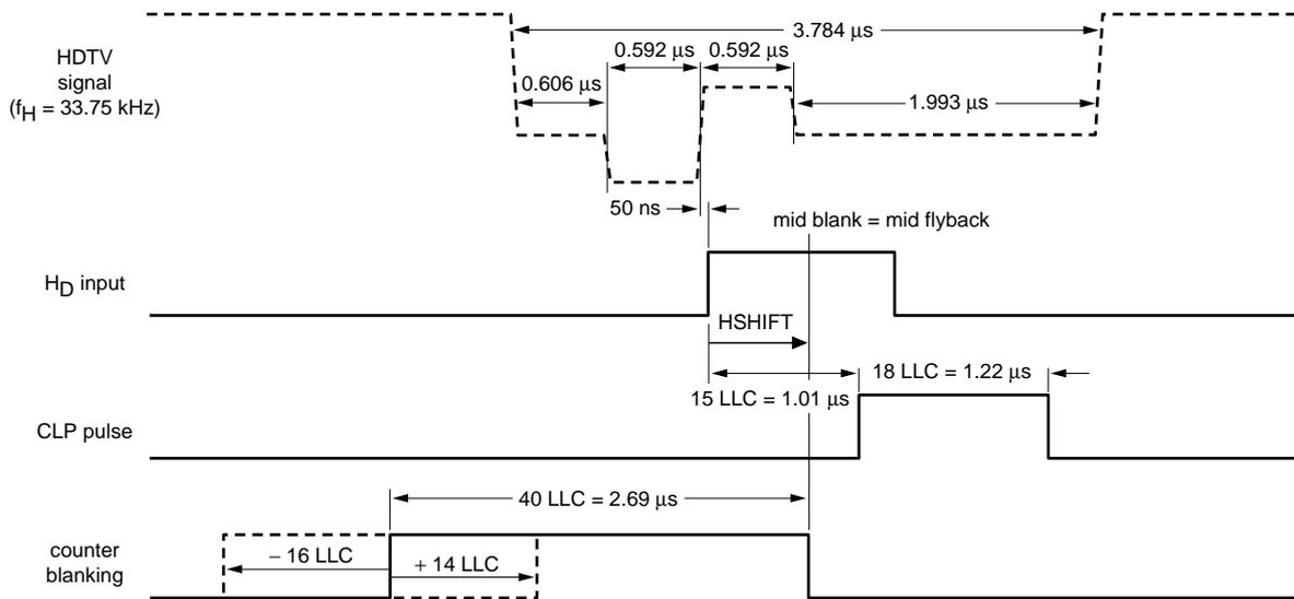
(b) Timing in HDTV mode (HDTV = 1, HDCL = 1)
