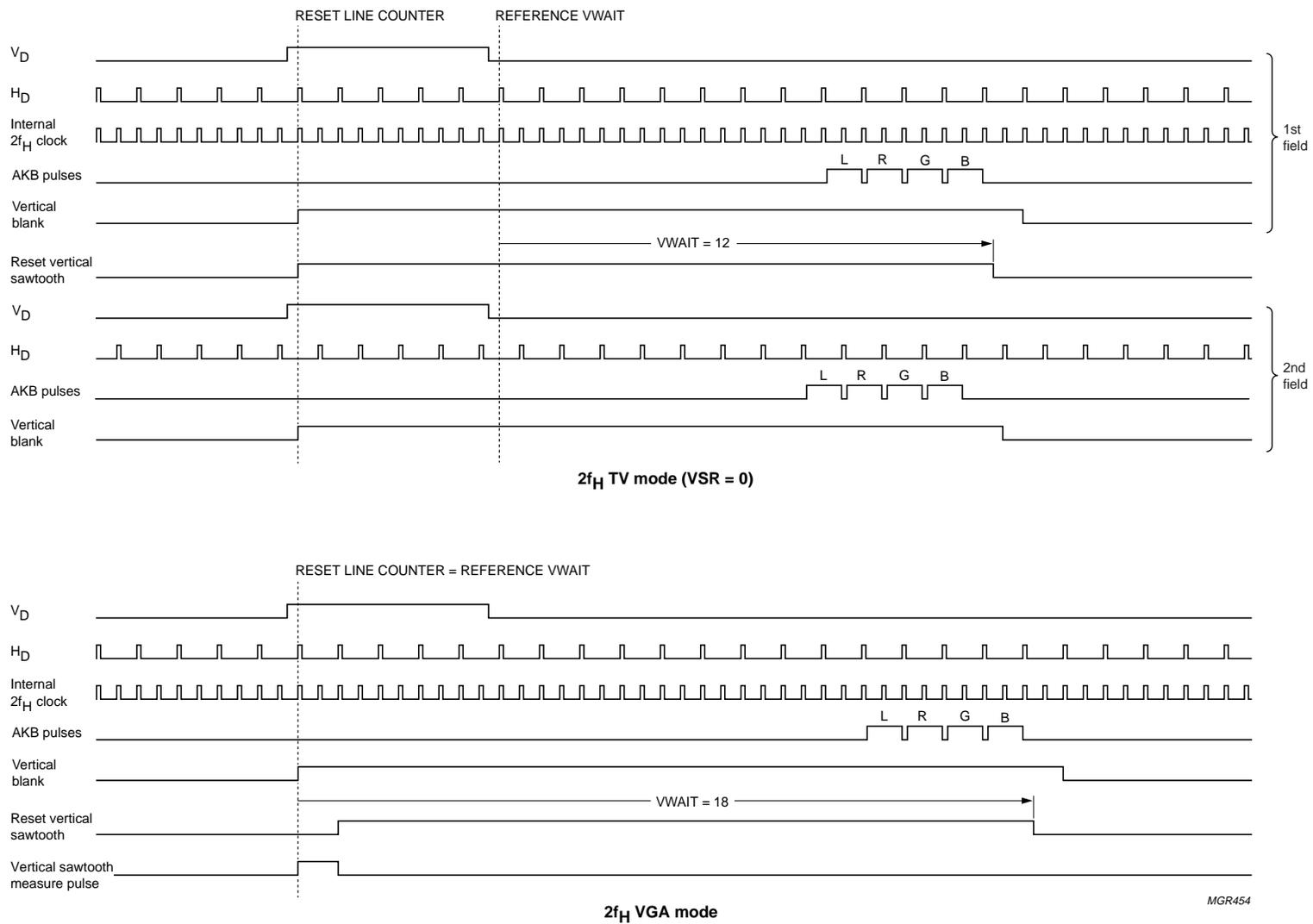
Fig.13 Vertical timing pulses for 2f<sub>H</sub> TV mode and VGA mode.
