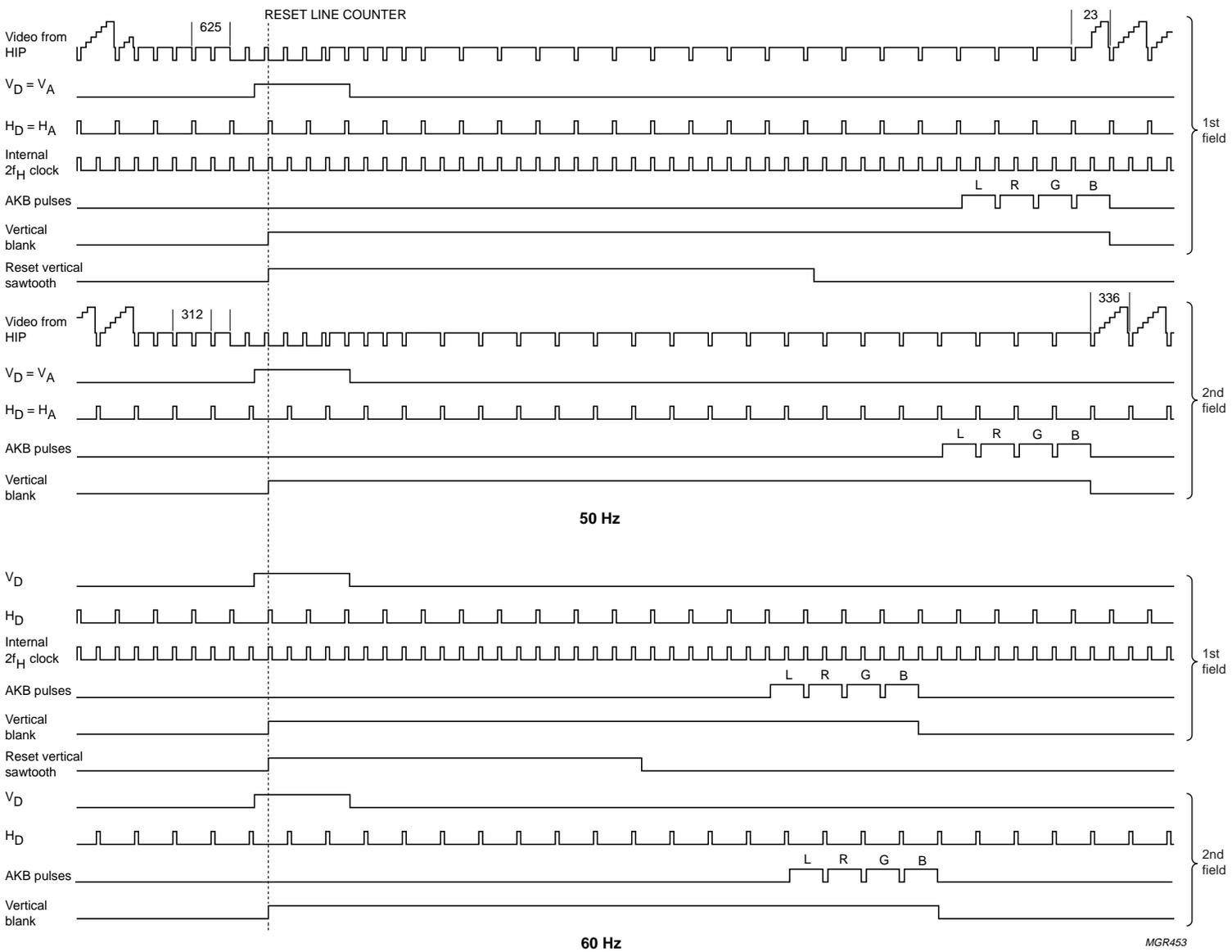
Fig.12 Vertical timing pulses for 1f<sub>H</sub> TV mode.
