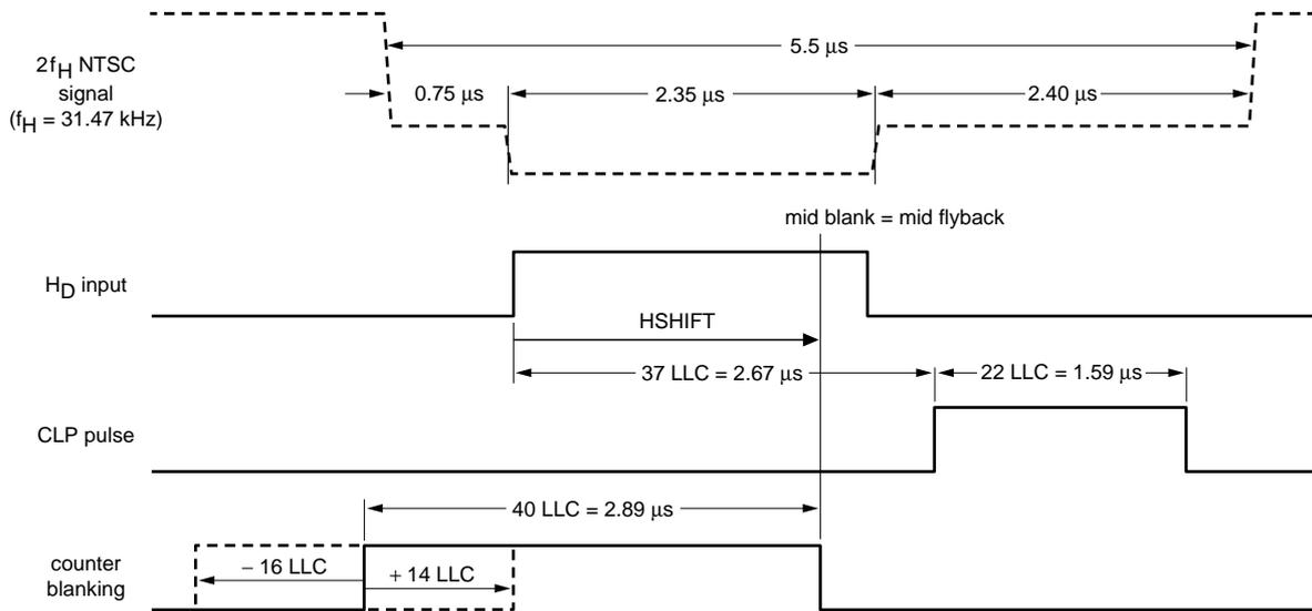
(a) Timing in 2f<sub>H</sub> TV mode (HDTV = 0, HDCL = 0)
