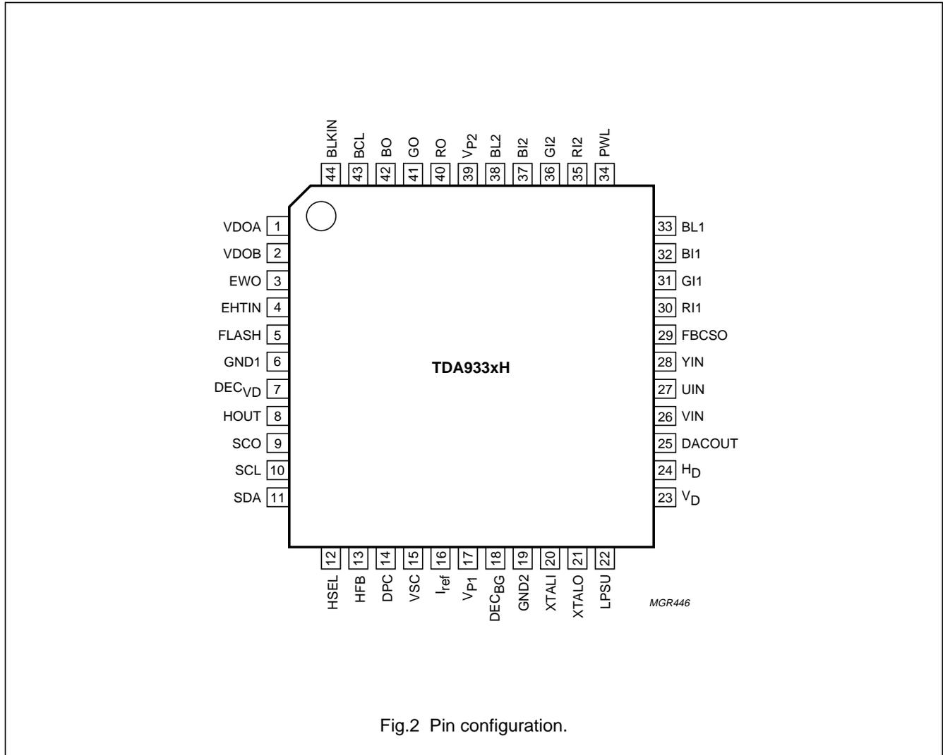
Fig.2 Pin configuration.
