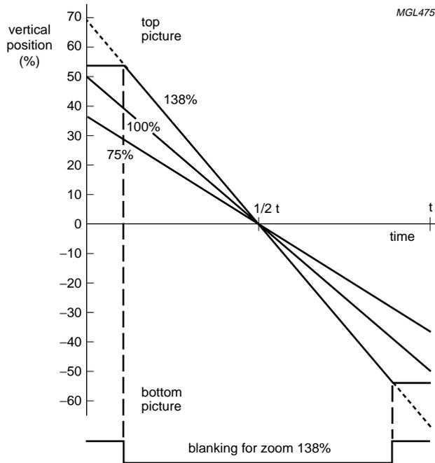
Fig.14 Vertical drive waveform and blanking pulse for different zoom factors.
